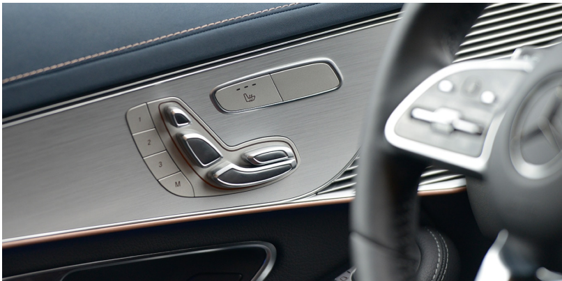
Figure 1-4. Seat controls in the 2020 Mercedes-Benz EQC 400 Prototype, informed by the mental model of a car seat (source: MotorTrend , 2018)
