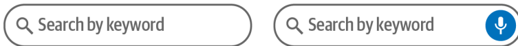
Figure 5-3. A progressively enhanced search component that provides a search box by default, and then voice support for devices that support voice recognition
