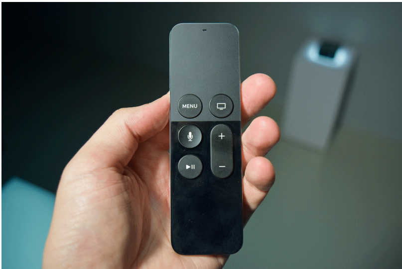
Figure 3-4. A smart TV remote, which simplifies the controls to only those absolutely necessary (source: Digital Trends, 2018)
