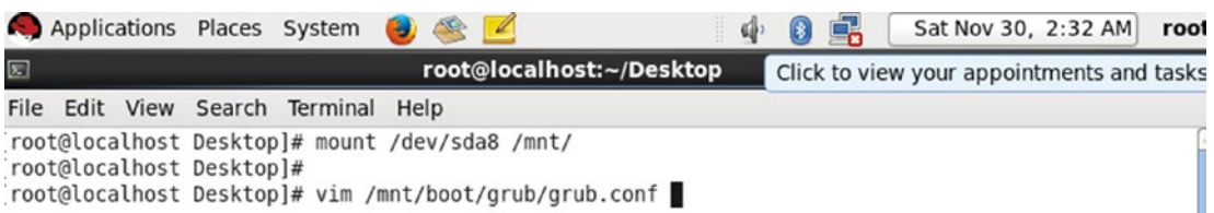
Figure 2-99. The mounting of Fedora’s partition
