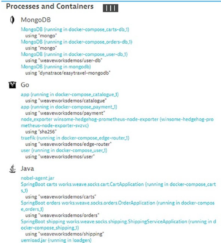
Figure 7-32. Dynatrace Kubernetes Processes and Containers view
