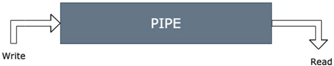
Figure 6-7. The architecture of an anonymous pipe
