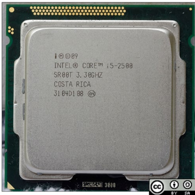
Figure 2-2. An Intel Core i5 processor may contain one, two, or four cores. Photo courtesy of Wikimedia Commons, CC by SA 4 International
