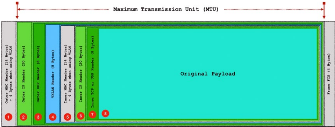
Figure 10-1. Format of a VXLAN packet
