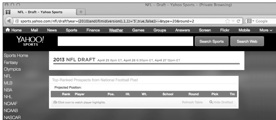
Figure 9-3: Yahoo! player search results were empty when the code checked whether the database version started with the number 5.
