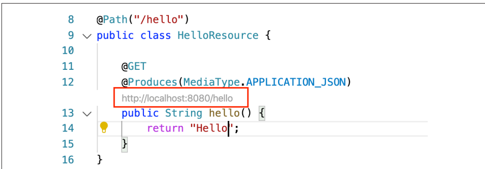
Figure 2-11. A clickable URL endpoint is generated by the VS Code extension for each endpoint method
