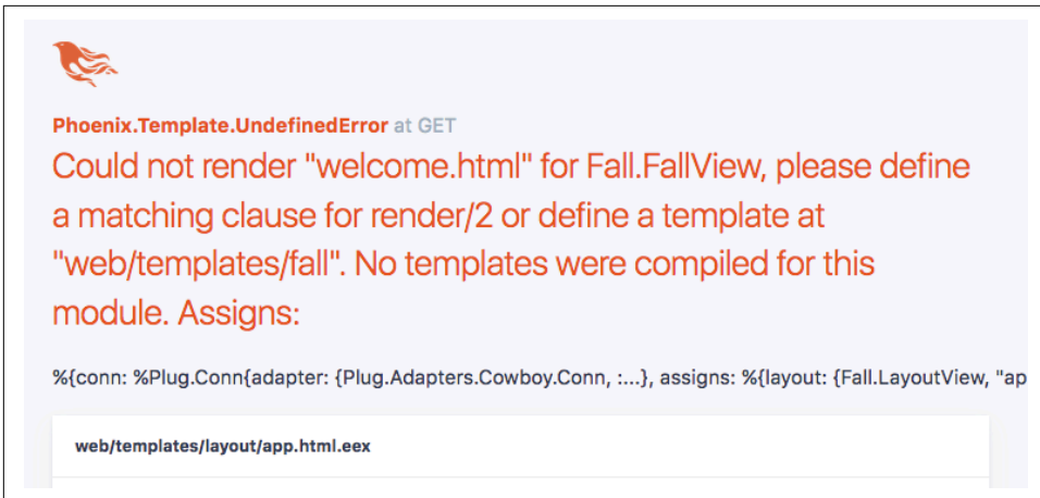
Figure 15-6. When a controller points to a nonexistent template
