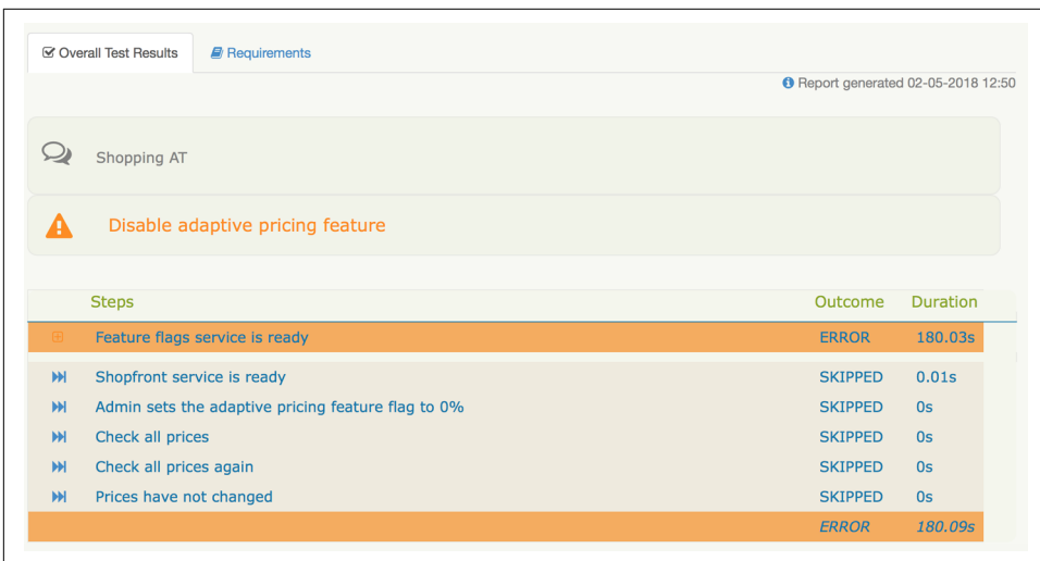
Figure 11-3. SerenityBDD's error report, showing steps that failed and steps that didn't run
