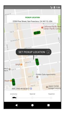
The main difference between the iOS and the Android version will be the map component. While iOS will use Apple maps by default, Android uses Google Maps. We will leave this setup as each platform has its own map component optimized, but it's good to know that we can switch the iOS version to use Google Maps just by configuring our component.
