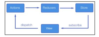
User triggers and **Actions** that are processed by **Reducers**, which are just pure functions applying changes to the state based on that **Action**. The resulting state is saved in a single **Store**, which is used by the **View** in our app to display the current state of the application.
