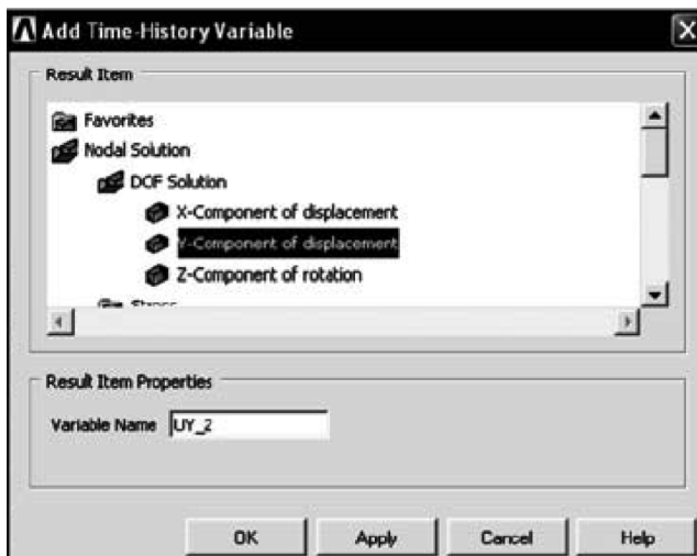
Figure 9.32. Selecting the displacement in y-direction.
