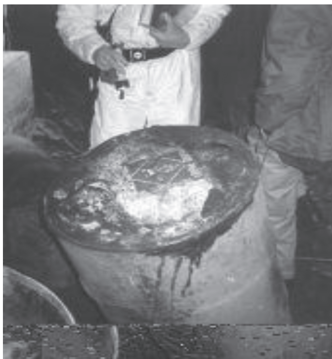
FIGURE 3.5 Bulging steel drum. (From Investigation Report No. 2002-02-I-NY, Figure 4, Page 20, U.S. Chemical Safety and Hazard Investigation Board, September 2003.)
