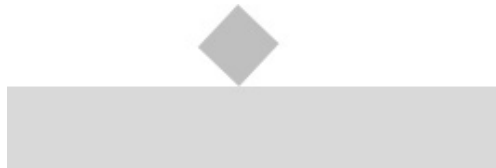
Figure 2.23: A block at tipping point
