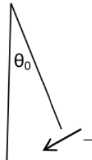
Figure 8.1: In the example the angle of the swing is measured counterclockwise from the vertical
