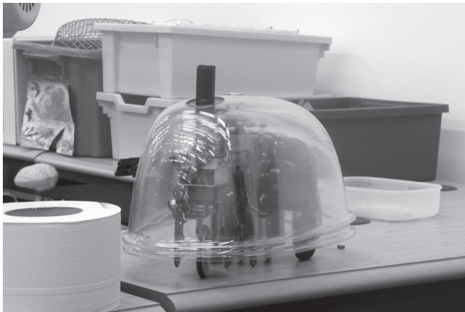
FIGURE 10.6 Grey Walter’s Tortoise, the First Recognized Robot
