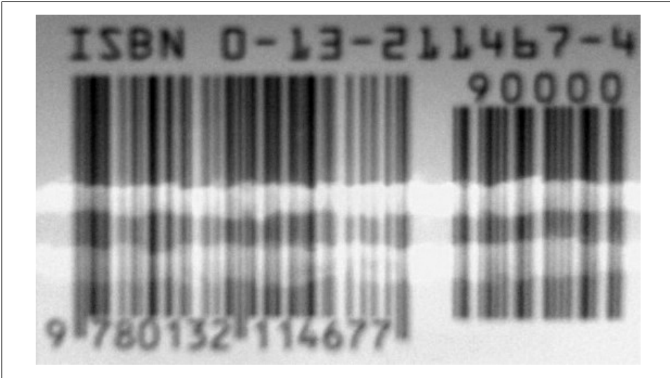
Figure 12-2. Barcode image blurred by being taken from inside the focal length of the camera lens, causing bars to run together
