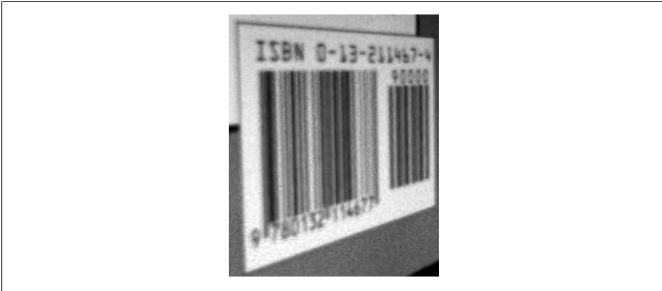
Figure 12-1. Barcode image distorted by perspective, due to photo being taken from an angle
