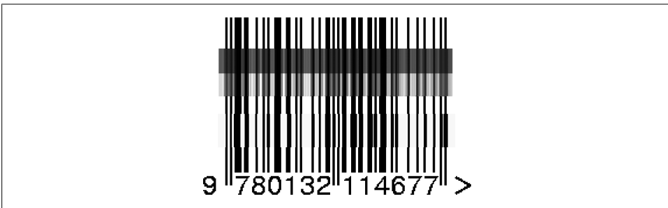
Figure 12-6. Photographic and generated images of barcode juxtaposed to illustrate the variation in bar brightness and resolution
