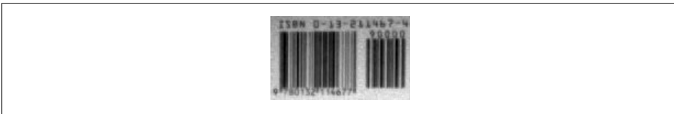
Figure 12-3. Barcode image contains insufficient detail, due to poor resolution of camera lens and CCD
