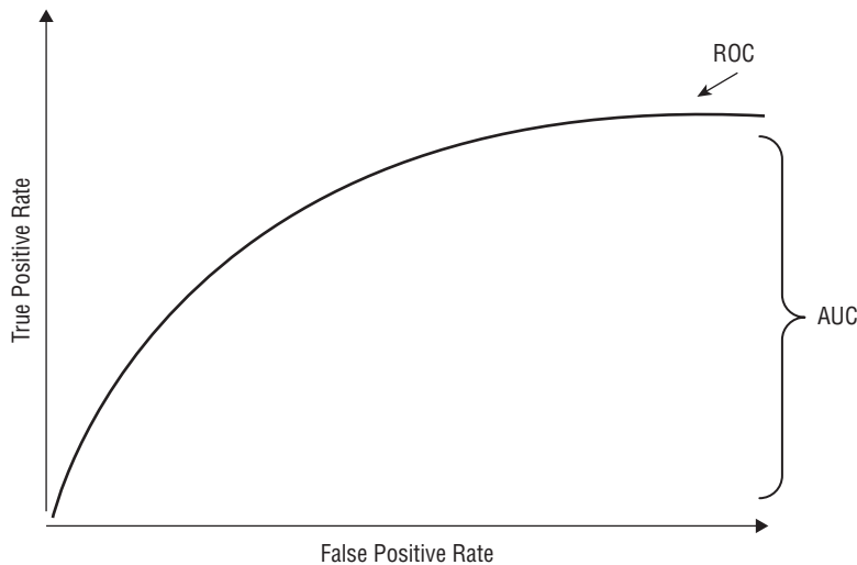
FIGURE 11.7 The ROC is the curved line, and the AUC is the area under that curve line.
