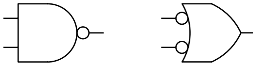
Figure 2-28: Redrawing a NAND gate using De Morgan's law
