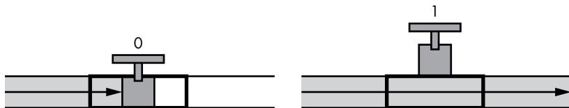
Figure 2-8: A water valve
