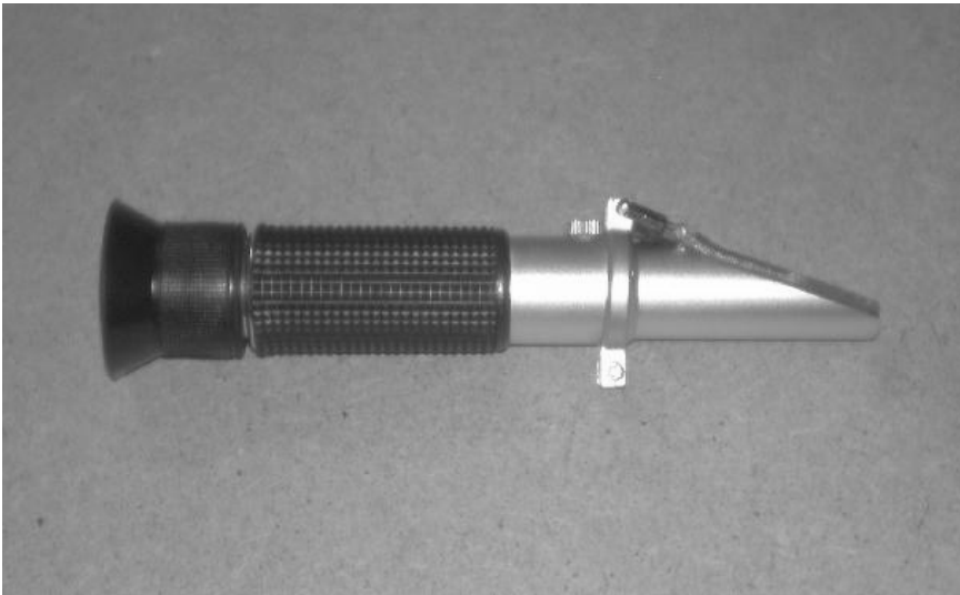
FIGURE 12.6 A refractometer. A small liquid sample goes under the plastic flap on the right, then a person looks through the eye-piece on the left.
