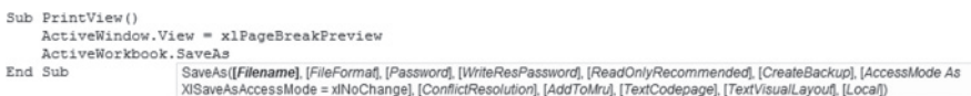
FIGURE 2.8 A tooltip displays a list of arguments utilized by a VBA method.
