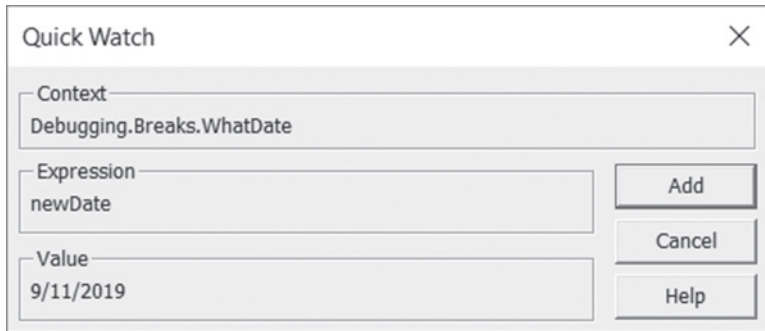
FIGURE 9.12 The Quick Watch dialog box shows the value of the selected expression in a VBA procedure.
