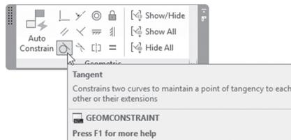
According to the AutoCAD definition, this constraint will constrain two curves to maintain a point of tangency to each other or their extension. You will see the following prompts:
