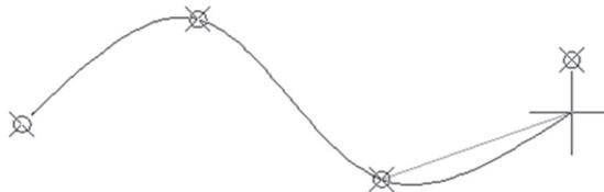
The user has the ability to specify tolerance for points other than the start and end points. See the following illustration:
