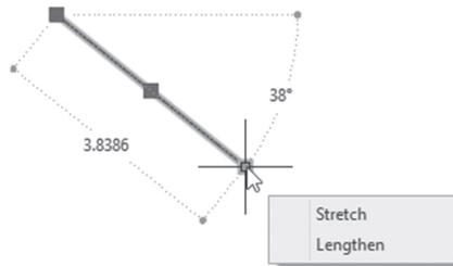
The two connected lines will show the two lengths and angles:
