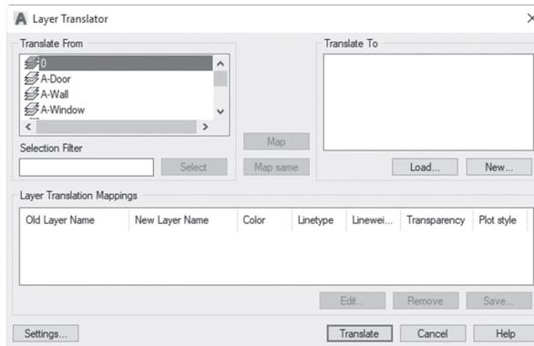
At the top left part, you can see the Translate From list, which contains the list of layers that need to be translated to your layering system. The Translate To list is empty due to the lack of your file. To load your file click the **Load** button; you can have DWG, DWT, and DWS files loaded.
