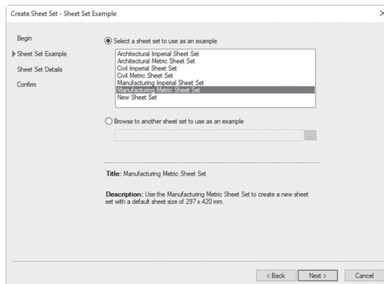
There are six examples: two for architectural (metric and imperial), two for civil (metric and imperial), and manufacturing (metric and imperial). These examples will contain only subsets using templates that are included
