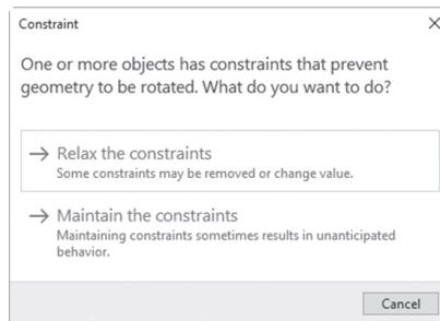
As you can see, AutoCAD will give you the choice either to relax the constraints or to maintain them. Selecting relaxing the constraint will mean removing only the associated constraint, which will allow the commands to be fulfilled.
