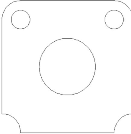
6. Using OSNAP and OTRACK (one point) draw the two circles at the right and left (distance center-to-center = 5.0, and Radius = 0.5)
