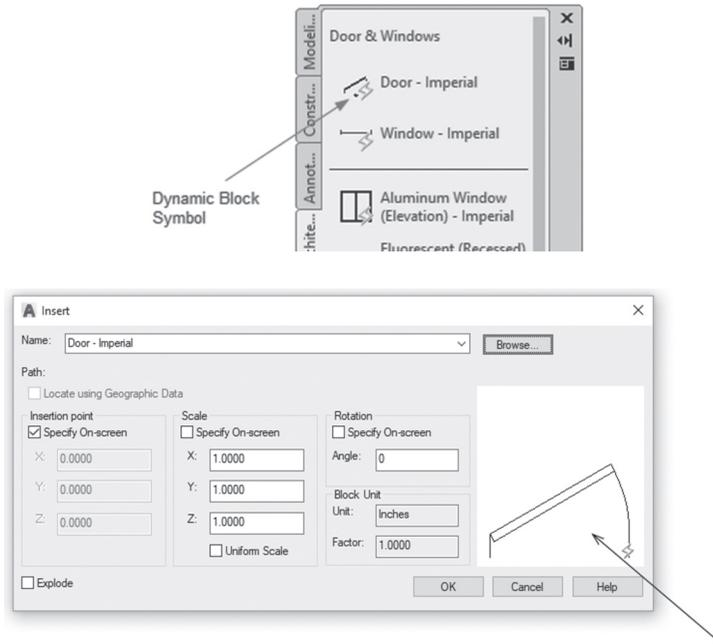
Dynamic blocks are very handy tools to help you to finish drawing production faster and with less mistakes, reducing the number of blocks to work with.
