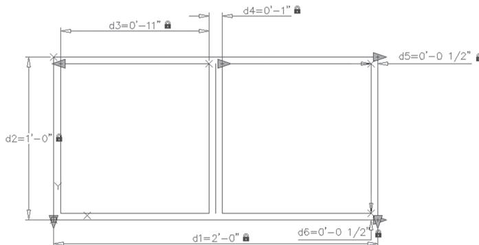
6. Using the **Parameters Manager**, make the following changes to the names: d1=Width, d2=Height, and d3=Glazing
