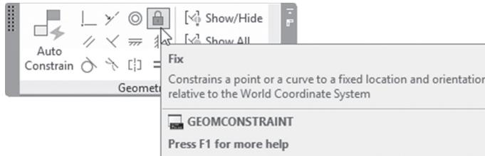
According to the AutoCAD definition, this constraint will constrain a point or a curve to a fixed location and orientation relative to the World Coordinate System. You will see the following prompt:
