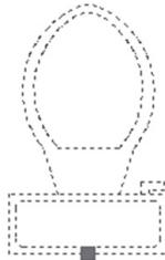
The whole block is one unit, and only one grip, the insertion point, is highlighted. There is a specific OSNAP to snap at this point called Insertion (or insert depending on where you are looking). Refer to the following illustration:
