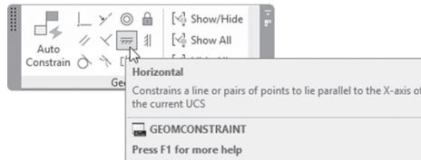
According to the AutoCAD definition, this constraint will constrain a line or pair of points to lie parallel to the X-axis of the current UCS. You will see the following prompts:
