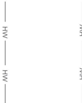
There is a system variable `PLINEREVERSEWIDTHS` will control whether to reverse the polyline width or not. If the value is 0 (zero) the polyline will not be reversed, but if the value is 1, the polyline width will be reversed. See the following illustration:
