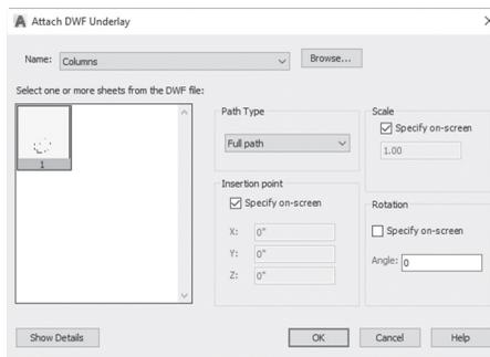
This dialog box is identical to the attaching DWG file dialog box except for the part for selecting which sheet of the DWF file you want to attach, that is, if you have a multiple sheet DWF file. AutoCAD permits to reference the same file more than once in the same drawing.
