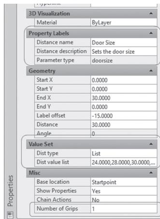
When you add a new parameter, AutoCAD will give it a temporary name, but as a user, you can change it to a proper name.
