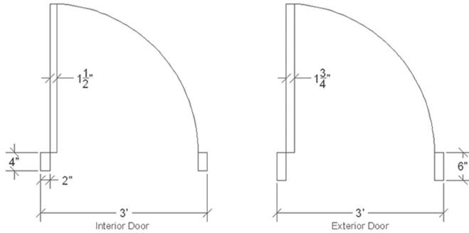
14. Create the following door blocks using the name beneath (the base point is the lower left point of the jamb):
