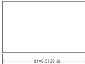
Using the Dimensional Constraint Settings dialog box, the user can choose to show/hide the lock symbol along with the showing the name.
