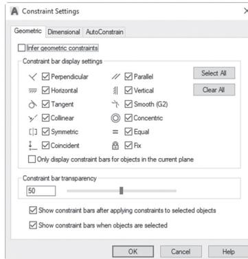
You will see that by default, all of the constraint will be displayed, and the user can select to hide any of the twelve constraints in the drawing. Also, control the following:
