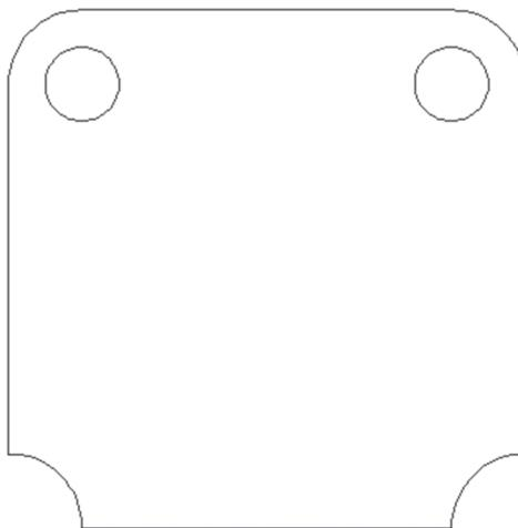
5. Using OSNAP and OTRACK (using two points), draw the circle at the center of the shape (Radius = 3.0)
