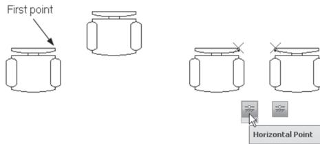
Note that although a polyline is considered a single object, if you use this constraint on it, AutoCAD will treat each object alone.
