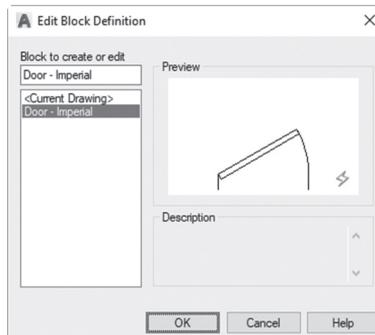
AutoCAD will show all the blocks in the current drawing; select the block by double-clicking, and simply click OK to go directly to the block editor to assess the desired features.
