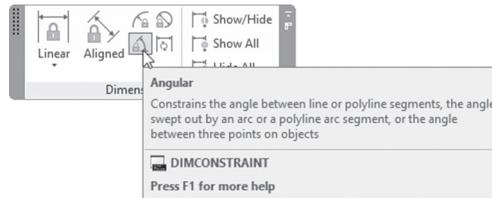
According to the AutoCAD definition, this Angular will constraint the angle between two lines or polyline objects, in an arc, or using three points. You will see the following prompts:
