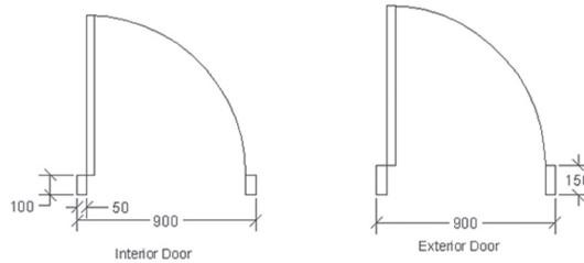
14. Create the following door block using the name beneath (base point is the lower left point of the jamb):
