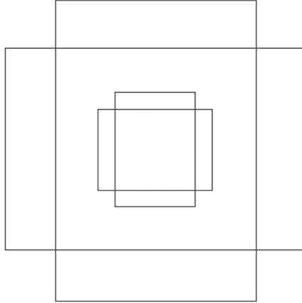
Specific objects like polylines will show more than the blue squares; they will show rectangles at the midpoint of each line and arc segment. The rectangles at the midpoint of the polyline have multiple functions. Depending on whether it is a line segment or an arc segment, AutoCAD will show a different menu. Go to the grip and stay for a second (don't click), and you will see the following:
