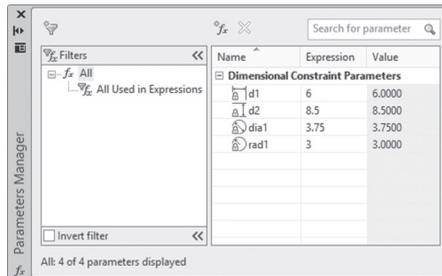
The Parameters Manager palette will be displayed showing all the existing Dimensional Constraint Parameters. As you can see AutoCAD is using the
