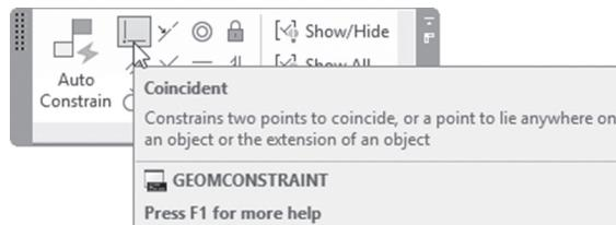
According to the AutoCAD definition this constraint will constrain two points to coincide, or a point to lie anywhere on an object or the extension of an object.
