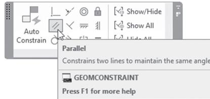
According to the AutoCAD definition, this constraint will constrain two lines to be parallel. You will see the following prompts:
