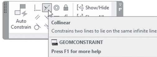
According to the AutoCAD definition, this constraint will constrain two lines to lie on the same infinite line.
