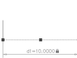
In the previous image, the Dimensional constraint was hidden, but when we selected the object, the Dimensional constraint appeared.
