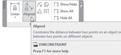
According to the AutoCAD definition, this constraint will constrain the distance between two points whether on the same objects or on different objects. You will see the following prompts:
