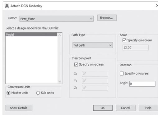
This dialog box is identical to DWG file except for one thing: the part about Conversion Units. If you know that MicroStation files deal with two units, Master and Sub, you have to tell AutoCAD whether the current AutoCAD unit is Master or Sub. AutoCAD permits reference to the same file more than once in the same drawing.
