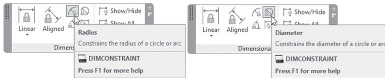
According to AutoCAD definition, these two constraints will constrain the radius or the diameter of a circle or arc. You will see the following prompts:
