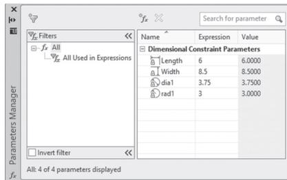
And user can create an equation including one or more of the parameters in the following example:
