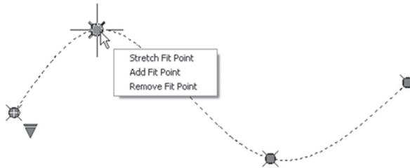
This menu will Stretch the current fit point, add a new fit point, or remove the current fit point. You will see an extra option if you stay at the start or end point of the spline, Tangent Direction, which will change the tangent direction of the spline.
