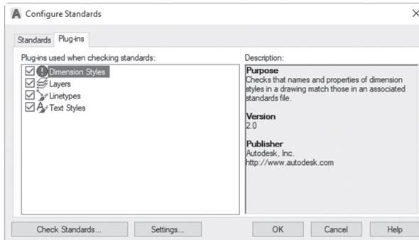
As said before, AutoCAD can check for five things only: Dimension styles, Layers, Linetypes, Multileader styles, and Text styles. To have full
