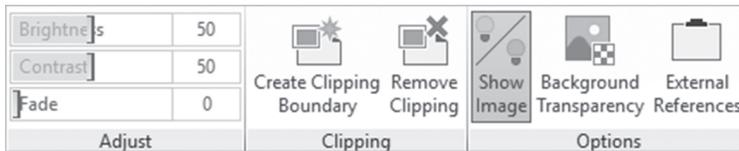
The Adjust panel contains Brightness, Contrast, and Fade slider, to control the image colors; the Clipping panel contains Create Clipping Boundary, and Remove Clipping buttons; finally the Options panel contains Show Image, Background Transparency (whether to show objects behind the image), and External References buttons.
