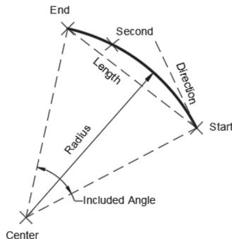
If you provide three of these eight pieces of information, AutoCAD will be able to draw an arc, but not with any three. The combination of the information needed can be found in the **Home** tab, using the **Draw** panel, while clicking the arrow near the **Arc** button to see all the available methods:
