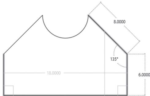
Keep moving and you will see more dimensions. The two rectangles at bottom right and left means  $90^\circ$  angles.
