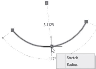
However, the endpoints of an arc will show the radius and the angle with the east, along with the Stretch and Lengthen commands:
