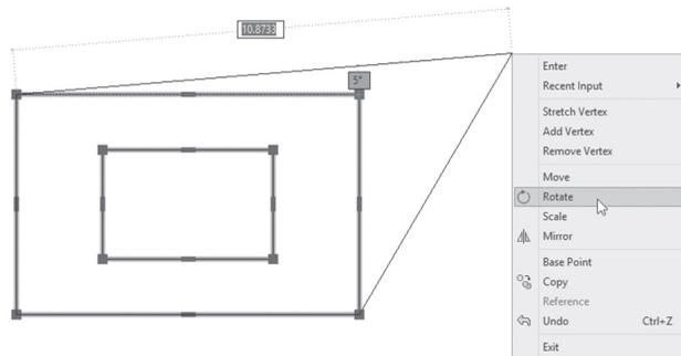
Now you can rotate the two shapes around the grip (this will be considered your base point), right-click again, and select the Base point option to select another base point, which will be the center of the two rectangles (using OSNAP and OTRACK):
