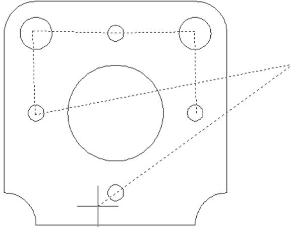
All the circles are selected because they are touched by the fence. The vertical line at the right will be selected as well. You can see that the fence lines are crossed which is 100% acceptable in AutoCAD.
