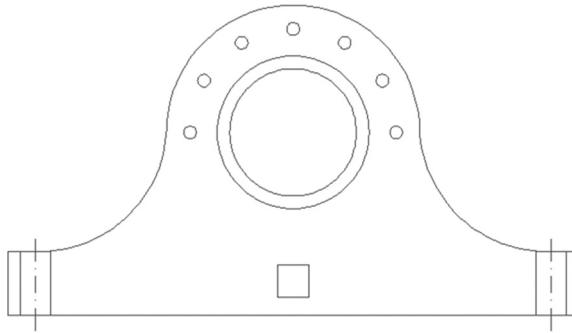
7. Select the polyline below the two big circles. Convert the top horizontal line to an arc by moving up distance = 0.25
