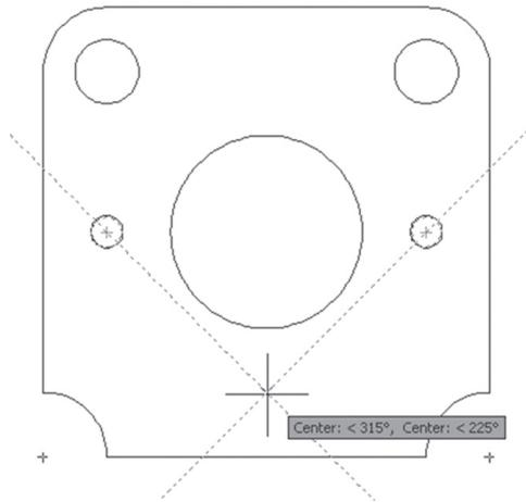
8. Do the same procedure to draw a circle at the top, to end up with the final shape as follows:
