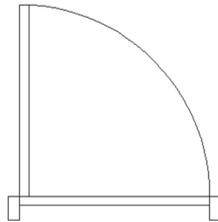
11. Add a Visibility parameter, selecting the upper left part of the door to be the location of the parameter. Note how the Visibility panel was turned on
