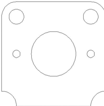
7. Change the increment angle in the Polar Tracking dialog box to 45. Make sure that **Track using all polar angle settings** is on, draw a circle (Radius = 0.5), its center specified using OSNAP, OTRACK, and polar tracking as shown below:
