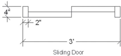
15. Create the following window blocks using the name beneath (base point is the lower left point of the jamb):
