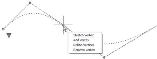
This menu will stretch the current vertex, add a vertex, or remove a vertex. The Refine Vertex option will replace the current vertex with two vertices:
