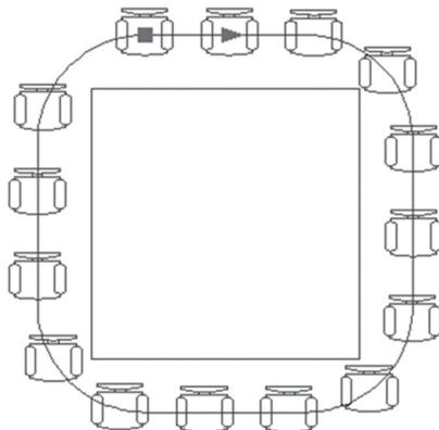
If you select the Divide option, AutoCAD will divide the path equally for all the objects, but if you select Measure, you should specify the distance between each object. The previous was produced by using Measure, the following by using Divide:
