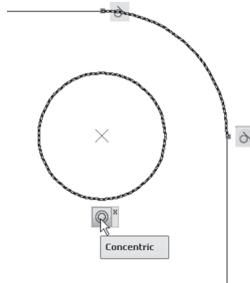
On the other hand, if you hover over an object with geometric constraint applied to it, Constraint Bars will highlight as well. Occasionally one object may hold more than one constraint, hence the bar will show more buttons.
