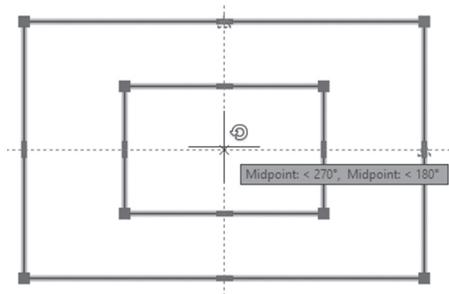
Right-click again and select the Copy option, to copy while rotating. Using Polar tracking specify an angle of 90, then press [Esc]. You will receive the following result:
