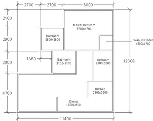
11. Create a 900 door opening as follows (you can always take 100 clearance from the wall). The main entrance, master bedroom, and walk-in closet door are at the middle of the wall:
