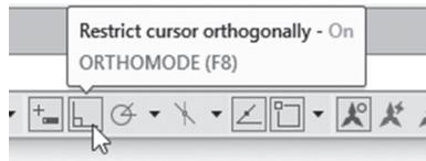
However, what if we want to use other angles such as 30, 45, 60, etc.? Ortho will not help in this case; for this reason AutoCAD introduced another function called Polar Tracking, which will show in the graphical area rays starting from the current point heading toward angles like 30, 45, etc. Since Ortho and Polar Tracking contradict each other, when you switch one
