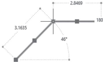
The midpoint of an arc will show the radius and the included angle along with two commands, Stretch and Radius:
