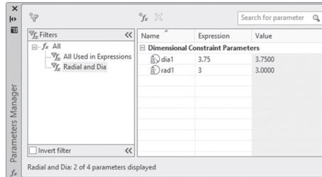
The user can easily differentiate between normal parameters and equations: equations starts with **fx**. The user can overwrite the equation by double-clicking it and inputting their own value.
