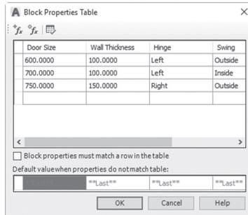
In order for these values to appear here, the user should go to the Properties palette of each dimensional constraint and add a list or increment.
