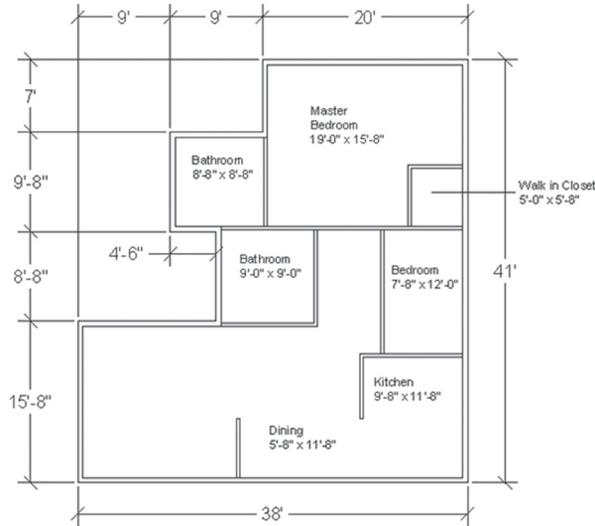
11. Create a 36" door opening as follows (you can always take 4" clearance from the wall). The main entrance, master bedroom, and walk-in closet door are at the middle of the wall:
