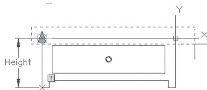
7. Add an Array action selecting the Height parameter, setting the distance to be 25
