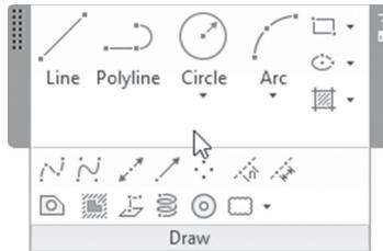
The button at the end of the tab names allows you to cycle through the different states of the ribbons. The main objective of this new feature is to give you yet more graphical area. Clicking the small button will produce the following:
