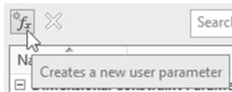
Input the name of the user-defined parameters, an expression (if valid); otherwise, input the current value. Later on you can include an expression involving dimensional constraint parameters. Refer to the example below:
