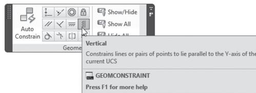
This command is identical to the Horizontal command allowing objects or points to be vertical.
