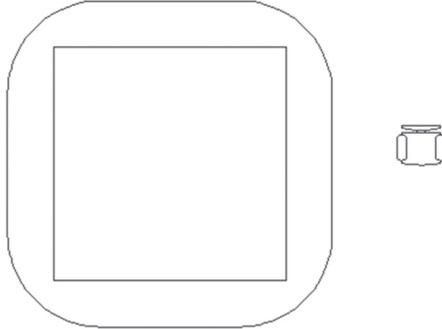
We will select the chair as the object to be arrayed and the outer polyline to be the path. See how AutoCAD will deal with this:
