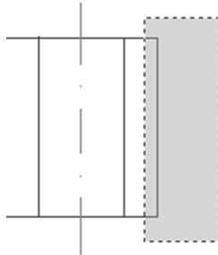
12. Hold the [Shift] key, select the lower right corner grip, and then select the upper right corner grip. Now release the [Shift] key, click any of the two grips, and go to the right by a distance equal to 0.25
