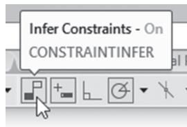
After you switch this checkbox on, AutoCAD will apply constraints to all objects as they are added to the drawing, using proper constraints depending on the object and the attached objects to it. Don't assume that this method is a replacement for the original method discussed at the beginning of this chapter, because you will be mistaken. This method will help you complete your work in fewer steps, that's all! Let's discuss the following example:
