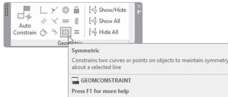
According to the AutoCAD definition, this constraint will constrain two curves or points on objects to maintain symmetry about a selected line. You will see the following prompts:
