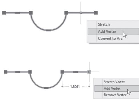
As you can see, you can Stretch the selected segment, add a vertex, convert a line to an arc, or convert an arc to a line.
