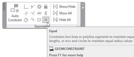
According to the AutoCAD definition, this constraint will constrain two lines or polyline segments to maintain equal lengths, arcs, or circles to maintain equal radius values. You will see the following prompts:
