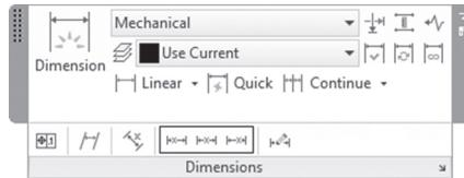
Each one of the functions will move the dimension text either to the left, center, or to the right. Refer to the following example (it moved it to the left):
