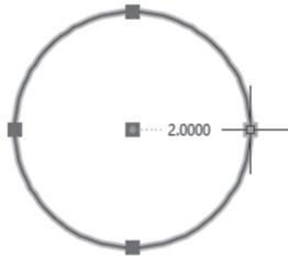
Shared endpoints between two segments of a polyline will show the length of the shared lines along with a shortcut menu which includes: Stretch Vertex, Add Vertex, and Remove Vertex.
