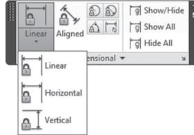
According to the AutoCAD definition, Linear will constrain either the horizontal or the vertical between two points (even if the two points form an angle other than 0, 90, 180, or 270). Horizontal command will constrain the X-axis distance between two points, and Vertical will constrain the Y-axis distance between two points. You will see the following prompt:
