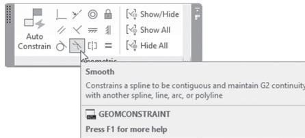
According to the AutoCAD definition, this constraint will constrain a spline to be contiguous and maintain G2 continuity with another spline, line, arc, or polyline. You will see the following prompts:
