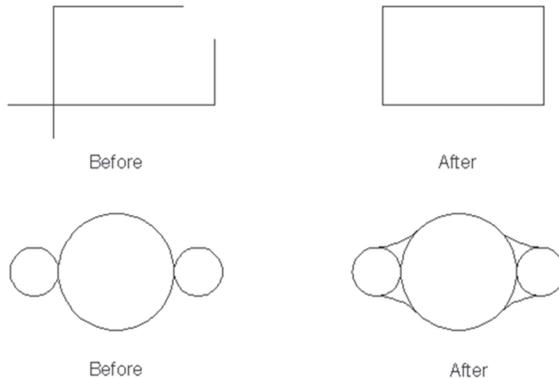
While working with a Radius greater than zero, the user can select between **Trim**, which will allow trimming to the original objects, or **No trim**, which will allow the original objects to stay as is. In both cases, the user will be able to see the arc when hovering over the second object, and can make sure that the value is correct!
