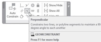
According to the AutoCAD definition, this constraint will constrain two lines or polyline segments to maintain a 90-degree angle to each other. You will see the following prompts:
