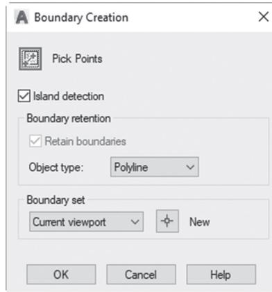
This command depends on a simple click inside the desired area in which you want to create a polyline. Therefore, we will start with the **Pick Points** button. When you are done, click OK to end the command, and create the polyline (or region) desired. You can move it (them) outside to calculate areas or any other desired commands. Meanwhile, you can make some amendments to the command to get different results; check the following options:
