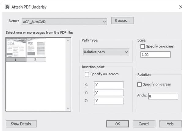
This dialog box is identical to the attaching DWG files dialog box except the part about selecting which sheet of the PDF file you want to attach, that is, if you have a multiple sheet PDF file. AutoCAD permits reference to the same file twice in the same drawing.
