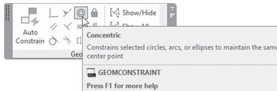
According to the AutoCAD definition, this constraint will constrain selected circles, arcs, or ellipses to have the same center point.
