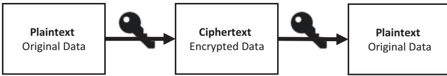
Figure 6-1. Symmetric encryption uses the same key for encryption and decryption
