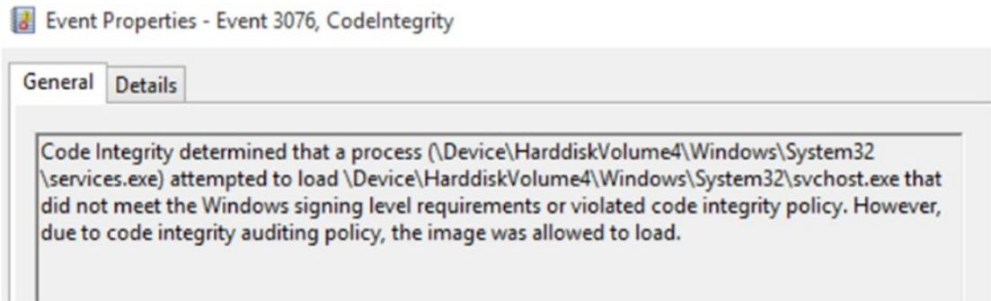
**Figure 3-5.** Event viewer showing a warning about the new application
