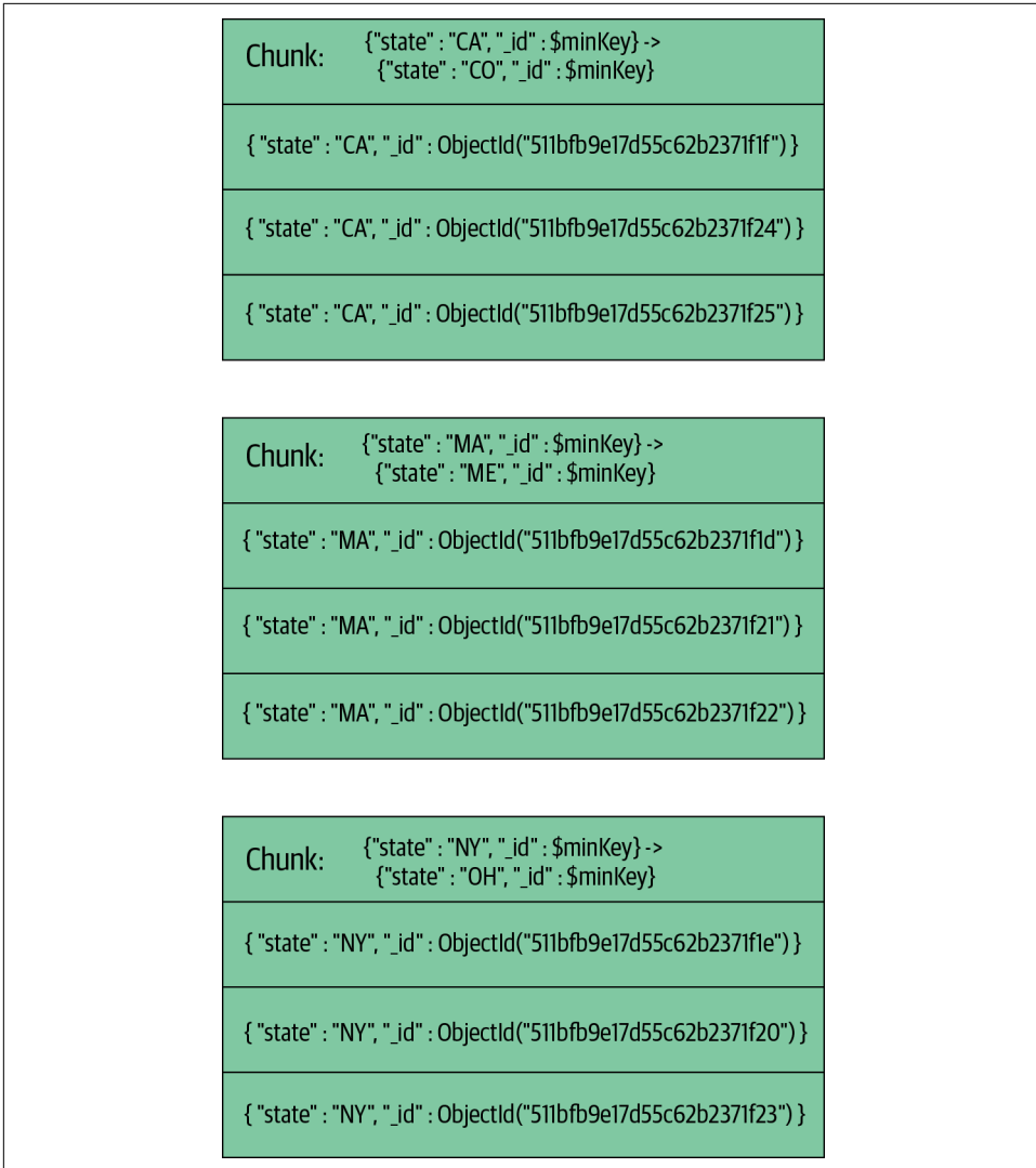
Figure 16-8. The inserted documents, split into chunks (note that, within each chunk, the “_id” values are increasing)
