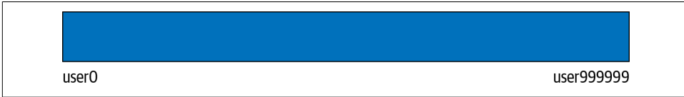
Figure 14-3. Before a collection is sharded, it can be thought of as a single chunk from the smallest value of the shard key to the largest
