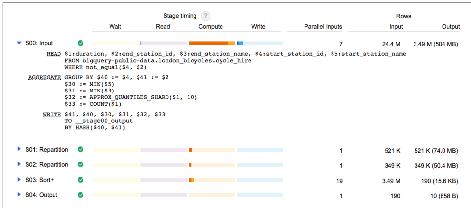
Figure 7-10. This query requires two repartition stages, but most of the time is spent in computation
