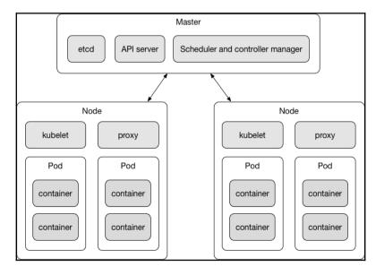
As you can see, the Kubernetes cluster consists of a Master node and a number of worker nodes with some components inside. While it may look scary and complicated at first glance, it will be easier to understand if we describe the concepts one by one, starting with the Pod.
