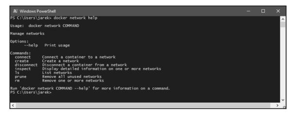
To have a detailed syntax and description of each option available for a specific command, use the -help switch for each of the commands. For example, to get the description of parameters available for docker network create, execute the docker network create -help.
