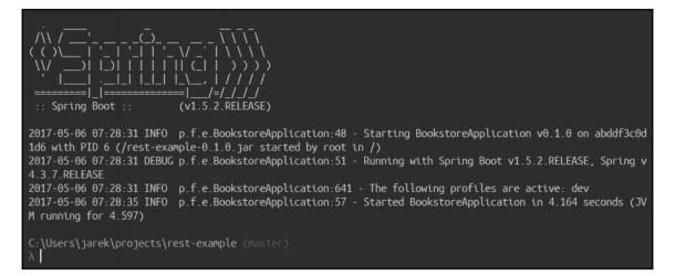
The -f flag acts as the same flag in Linux tail command, it will continuously display new log entries on the console. When you are done, hit CTRL + C to stop displaying log files on the console. Note that this is different from hitting CTRL + C when attached to the container, where CTRL + C would kill the process running within the container. This time, it will just stop displaying the log file and it's safe.
