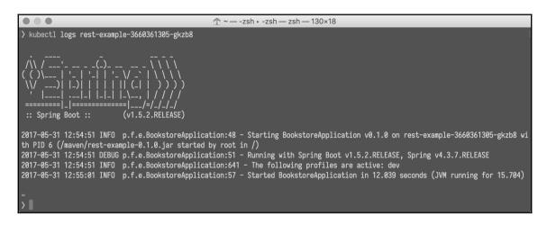
Viewing the log is not the only thing we can do with a specific Pod. Similar to Docker (a Pod is running Docker, actually), we can interact with a container by using the kubectl exec command. For example, to get a shell to the running container:
