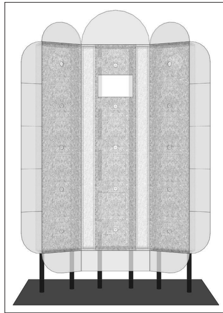
FIGURE 20-1: The design for the Magic Mirror, showing where the Raspberry Pi cameras (the small circles) are mounted in the mirror surfaces.
