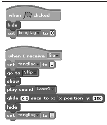
FIGURE 10-12: The final scripts for the fireball, including the firing flag.
