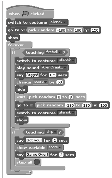
FIGURE 10-10: Setting up the alien and detecting when it's hit.
