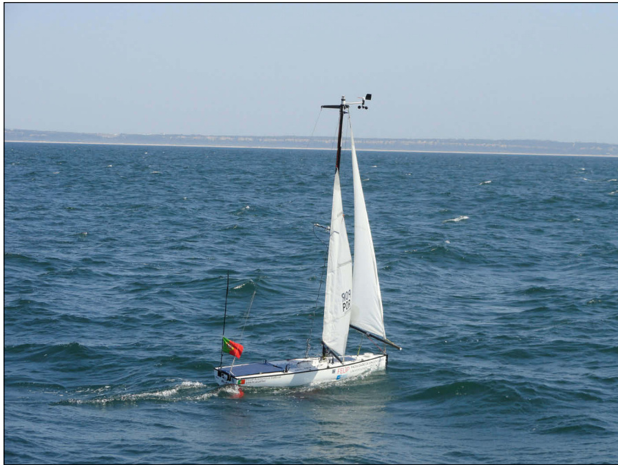
Figure 16-2: FASt, the autonomous sailboat.
