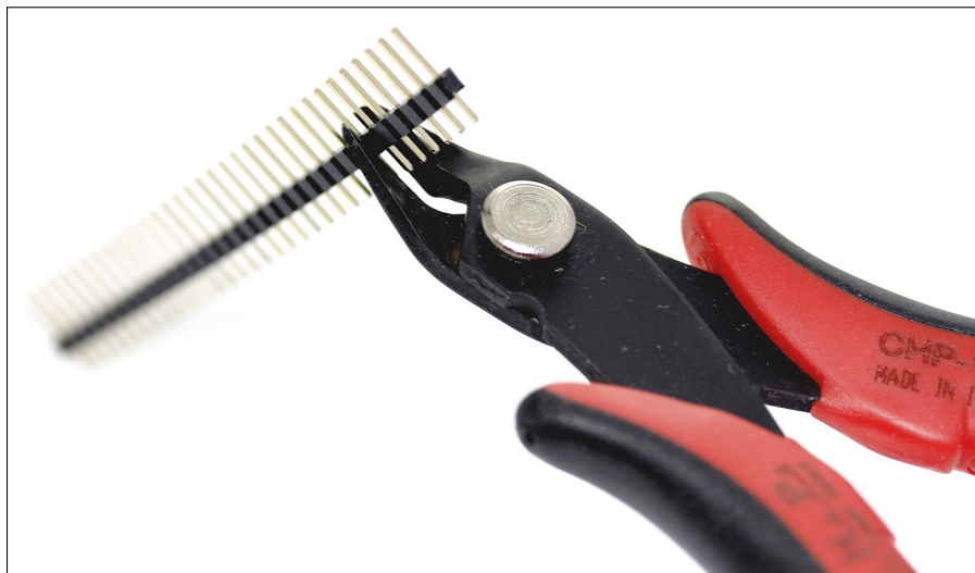
Figure 15-2: Cutting the headers to length.
