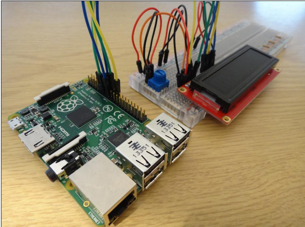
**FIGURE 10-3** Mounted LCD screen and potentiometer
