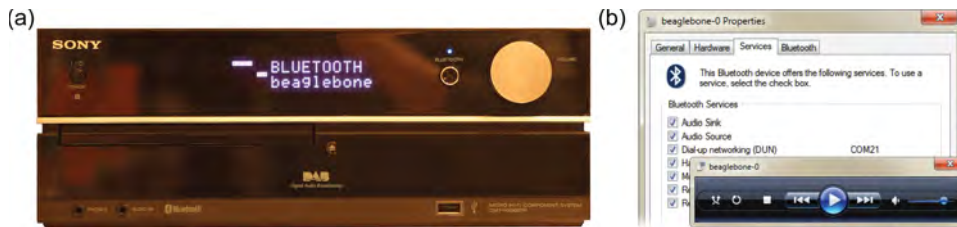
Figure 12-6: Bluetooth A2DP connections: (a) Sony Hi-Fi; (b) Windows machine via motherboard Bluetooth
