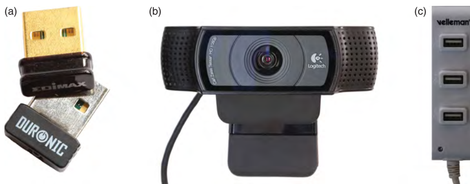
Figure 1-8: (a) USB Wi-Fi adapters; (b) the Logitech C920 camera; and (c) a Velleman USB hub (bus powered)
