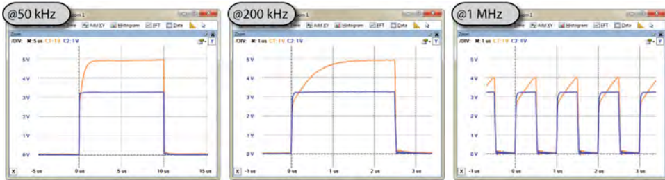
Figure 8-20: Switching BSS138-based translators from 3.3V to 5V logic levels at 50kHz, 200kHz, and 1MHz
