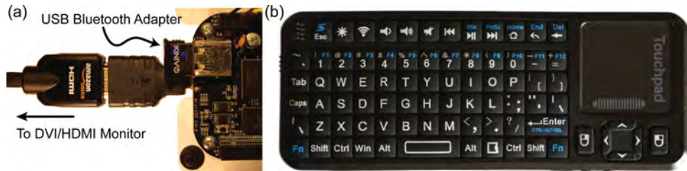
Figure 11-1: (a) Connection to an HDMI and a Bluetooth adapter (b) a Bluetooth keyboard/touchpad
