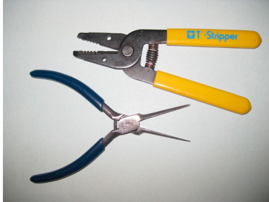
Figure 2-4: A gauged wire stripper/cutter and needle-nose pliers.
