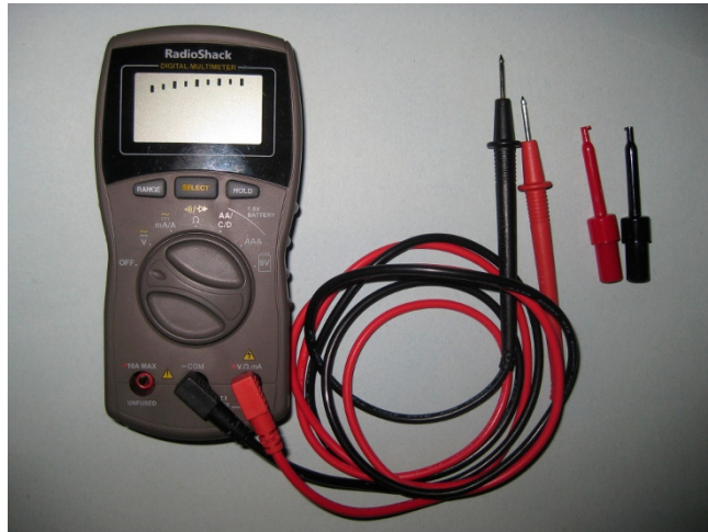
Figure 2-1: A multimeter and spring-loaded test clips.
