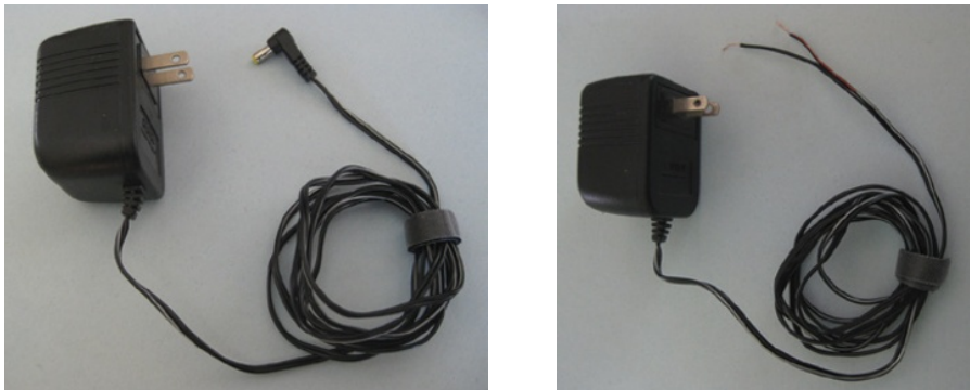
Figure 12-6: This AC adapter converts 120 volts AC to 7.5 volts DC and supplies up to 300 mA of current. I modified the output of this adapter to make it easier to use in DC circuits.
