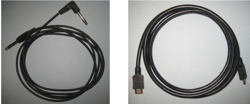
Figure 12-2: An analog audio cable (left) and an HDMI cable (right) facilitate the transmission of information between two pieces of electronic equipment.
