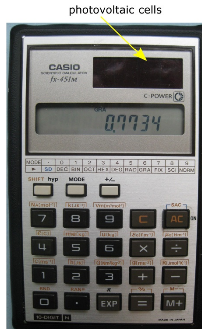
Figure 1-8: This calculator is powered by photovoltaic cells.
