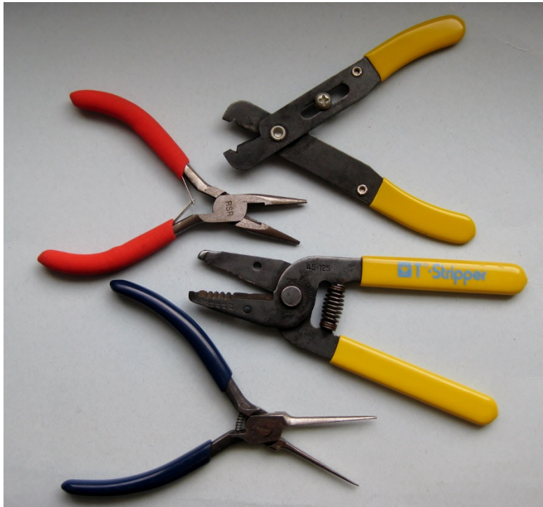
Figure 15-3: Tools of the trade (top to bottom): wire cutter/stripper, mini needle-nose pliers, wire stripper, needle-nose pliers.
