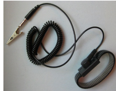
Figure 2-5: An antistatic wrist strap can prevent you from zapping sensitive components.
