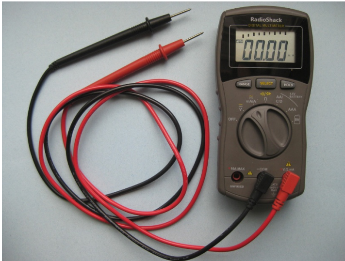
Figure 16-1: Multimeters measure voltage, resistance, current, and continuity.
