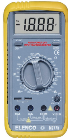
Figure 13-1: Multimeters measure voltage, resistance, and current.
