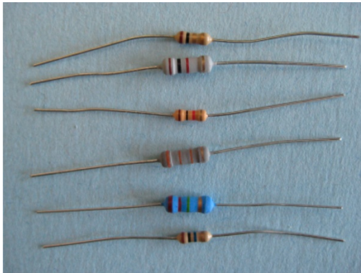
Figure 5-1: Resistors come in a variety of sizes and resistance values.
