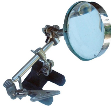
Figure 13-4: These helping hands combine alligator clips with a magnifying glass.
