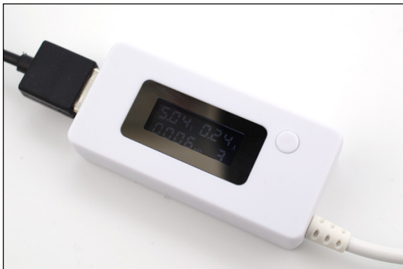
FIGURE 4-1: A USB power meter, reading the power flowing into a Raspberry Pi 2
