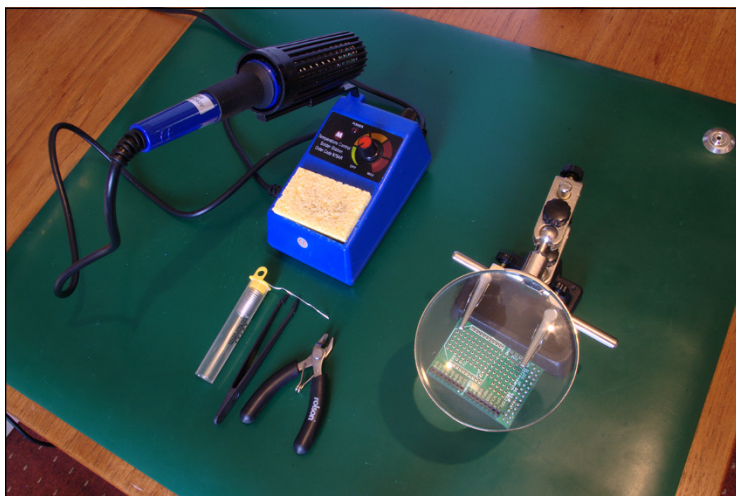
FIGURE 13-4: An example soldering work area with a protective antistatic workmat
