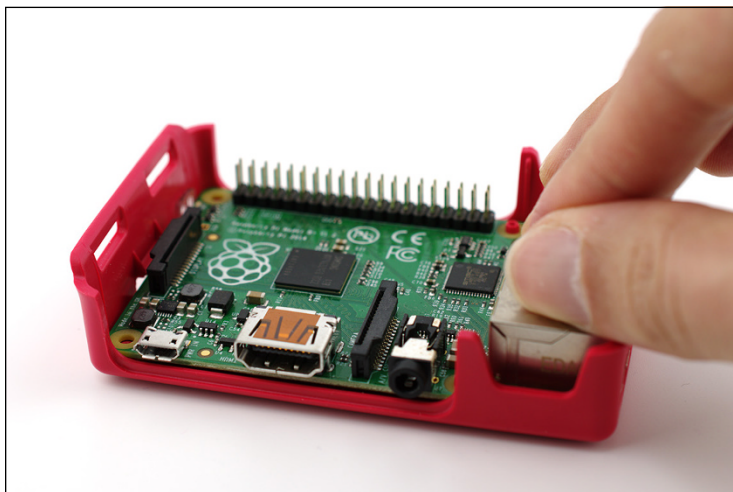
FIGURE 16-2: Mounting the Raspberry Pi inside the official case
