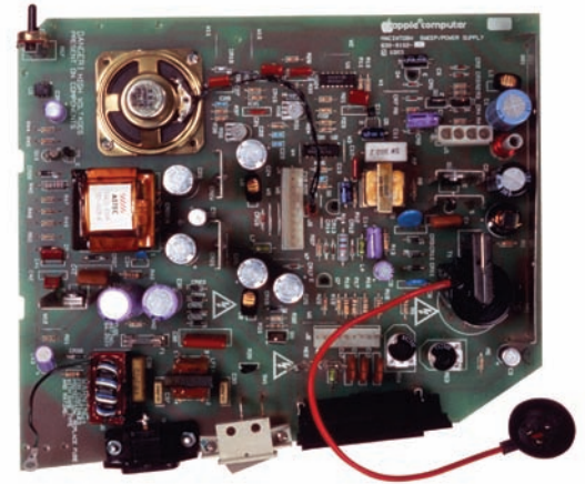
The Macintosh analog board, which contains the power supply and video generation circuitry
