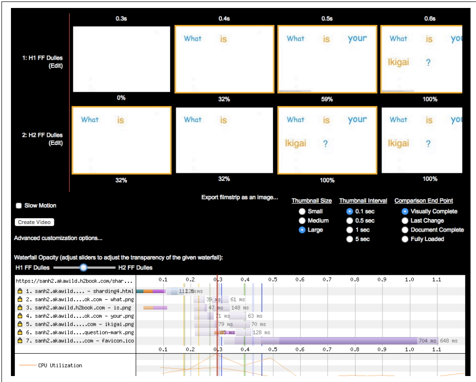
Figure 6-8. WPT filmstrip and timeline comparing loading a page that uses two hostname shards on h1 versus h2
