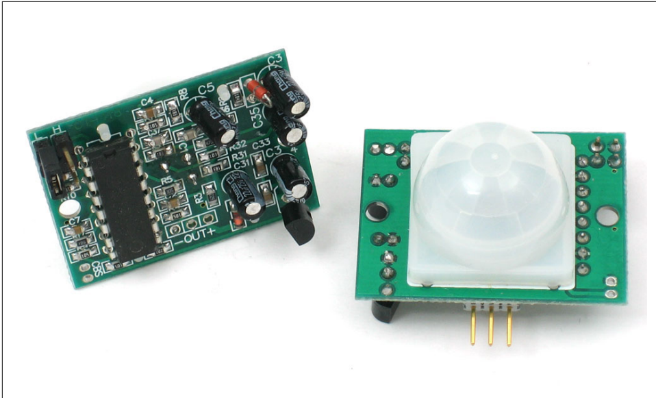
Figure 6-1. PIR Sensor - Photo Creative Commons, Adafruit Learning Systems
