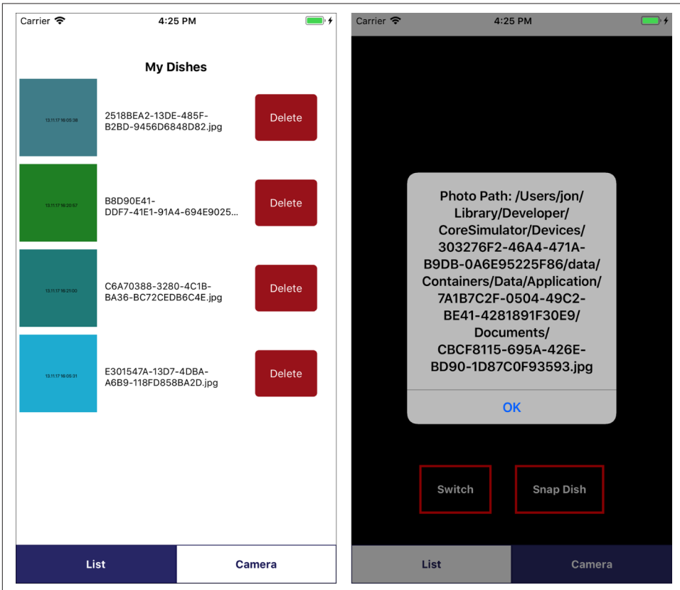
Figure 4-6. The App.js now includes a bottom toggle for page switching; CameraContainer and ListContainer are loaded interchangeably
