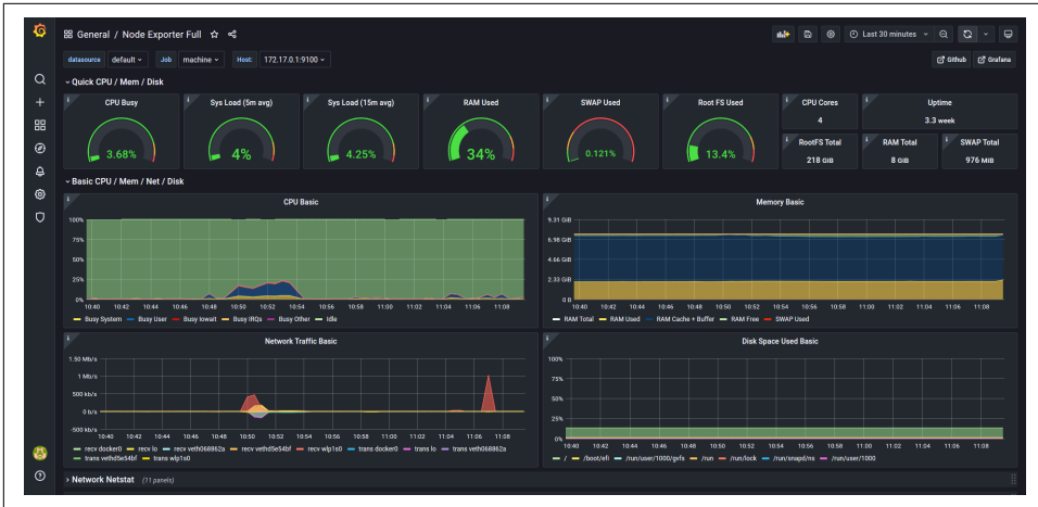
Figure 8-8. A screenshot of the Grafana UI with the Node Exporter Full dashboard
