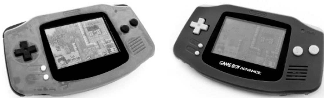
Figure 6.1 A built-to-order Retro Modding GBA that cannibalizes the AGS-101's backlit screen (left) beside an unmodded 2001 model with its default dim screen (right). Both display the same scene in FE7 .
