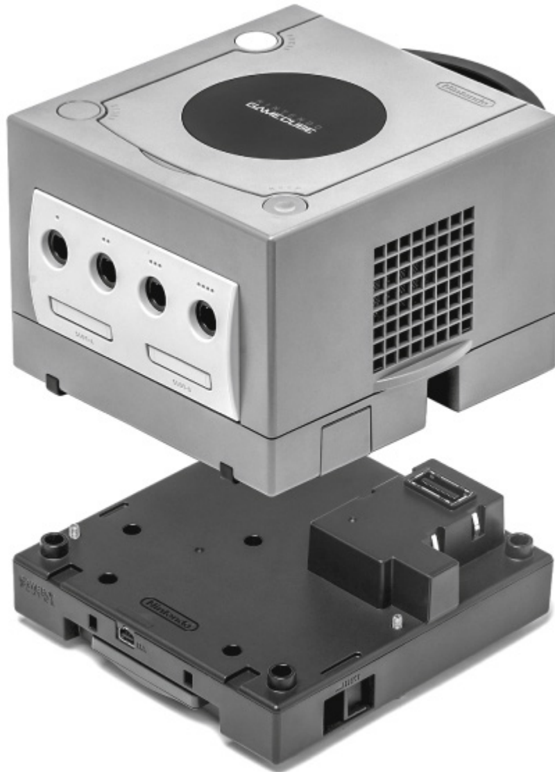
Figure 3.1 The GBP, with a GBA game inserted, ready to attach to the GameCube via a high-speed parallel port. Photo by Evan Amos, Wikimedia Commons.
