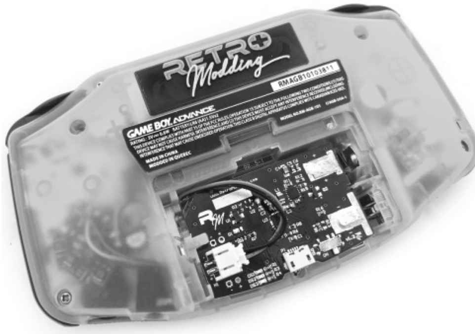
Figure 6.2 The back of Retro Modding's GBA, showing the custom USB-rechargeable battery back and the company's logo where the barcode used to be. The transparency of the shell simulates an aesthetic of technical mastery.
