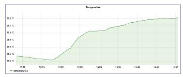
Once you have the time-series graph set up how you like, you can go ahead and duplicate it to plot the CO2 and TVOC levels. While the stat and gauge visuals only show the last non-null value, the time-series graphs will plot all the persisted data points within the selected time range. You can customize the visible time window by selecting the desired range in the drop-down menu in the upper-right corner.
