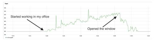
In my particular instance, I had my sensor hub in my office while writing this chapter and was observing the CO2 levels that the SGP30 sensor was measuring. It was interesting to see that while I was in my office without the window open, the CO2 levels were increasing at a regular rate. As soon as I opened the office window, it only took about five minutes for the CO2 PPM measurement to drop by almost 100 points. Feel free to explore and investigate
