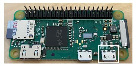
With that MicroUSB port only providing power to the device, we'll be able to check and see whether the wireless network is configured properly. You can
