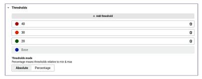
You can set the color for each threshold by clicking the colored circle and selecting a color for that threshold. Also be sure to set the Min to 0, Max to 50, and Show threshold labels to enabled. With that done, you should have a gauge that looks something like this:
