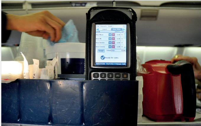
A portable point-of-sale terminal with a resistive screen, as currently used by an airline. The stylus is stowed at the top.
