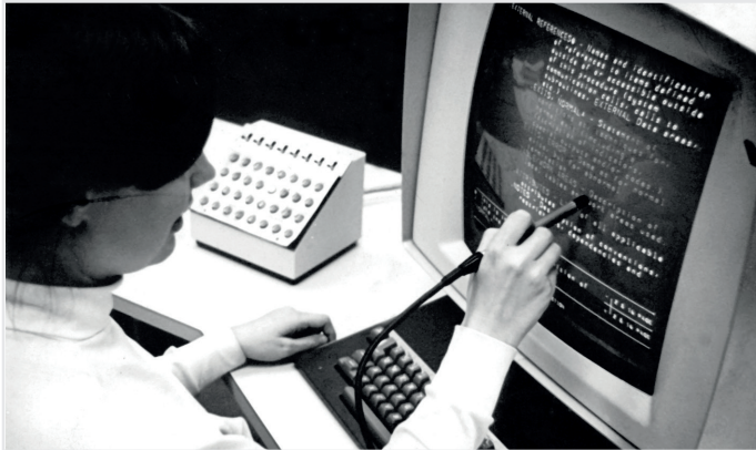
Using a pen to select text with the Hypertext Editing System on a computer terminal located at Brown University in 1969.
