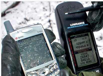
A resistive touch smartphone and passive stylus covered in snow, but still being successfully used to log data (c.2007).
