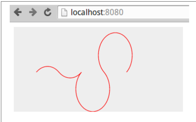
Figure 4-14. Changing the elliptic-arc flags
