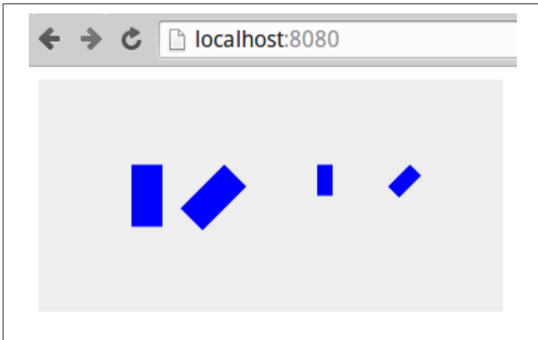
Figure 4-15. Some SVG transforms: rotate(45), scale(0.5), scale(0.5), then rotate(45)
