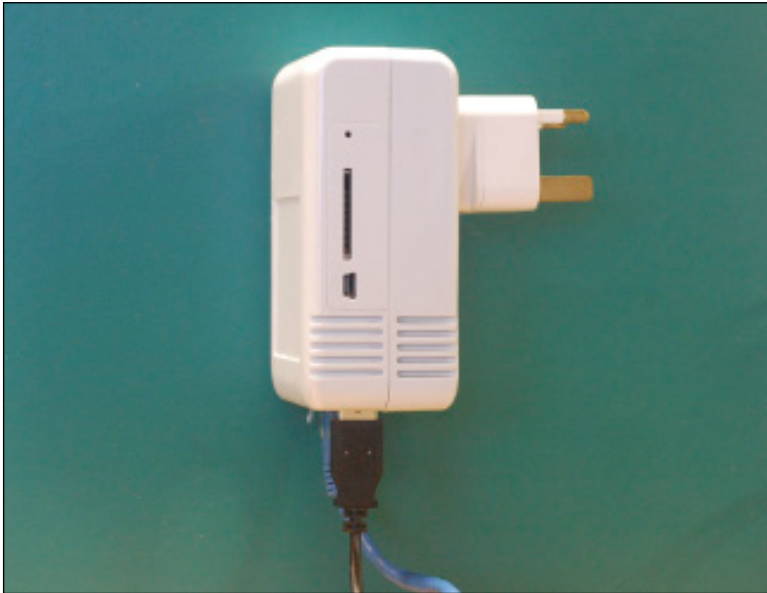
A SheevaPlug, looking more like a power adapter than a tiny computer.
