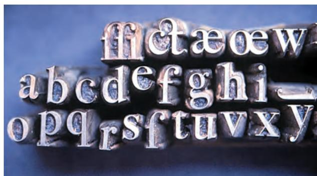
Figure 1–12 Actual Bodoni punches. Carved punches were driven into other pieces of metal called matrices. Molten metal was then poured into these matrices, making the actual type. Courtesy of Summer Stone.
