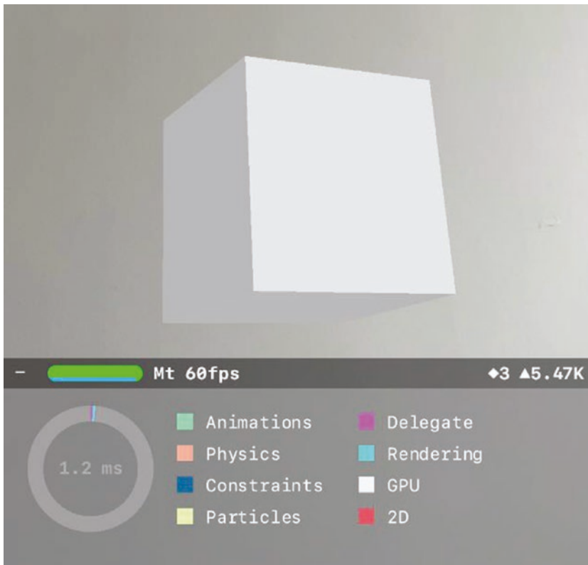
Figure 4-3. Showing Statistics gives information about how much effort the scene is taking to render
