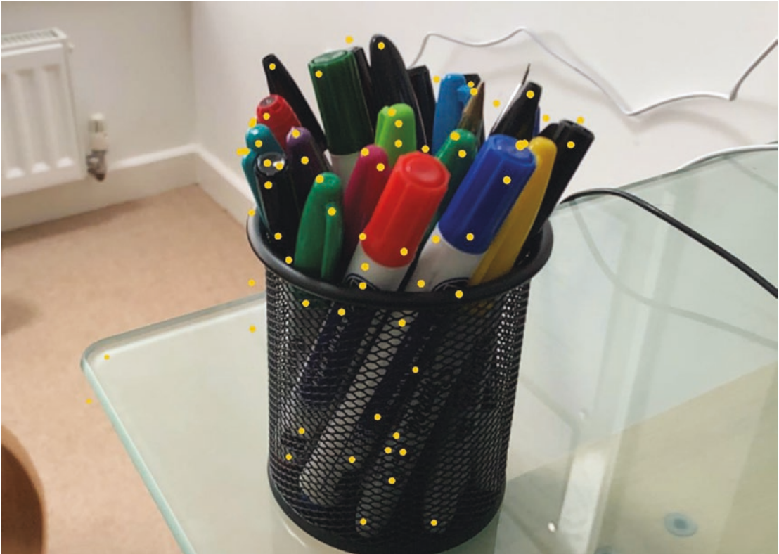
Figure 4-1. Showing feature points in a scene helps us understand how the app is looking for points of interest in the scene
