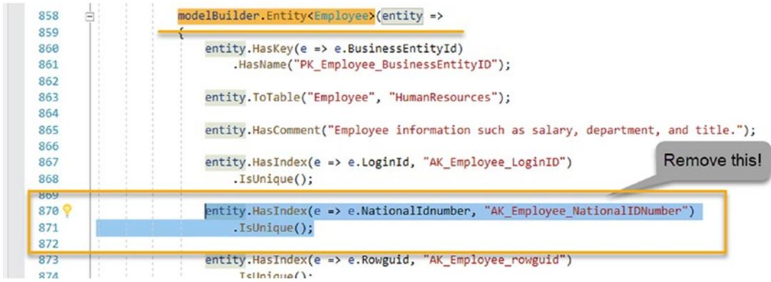
**Figure 10-30.** Remove the Employee Fluent API code for creating the index that was dropped in the previous migration
