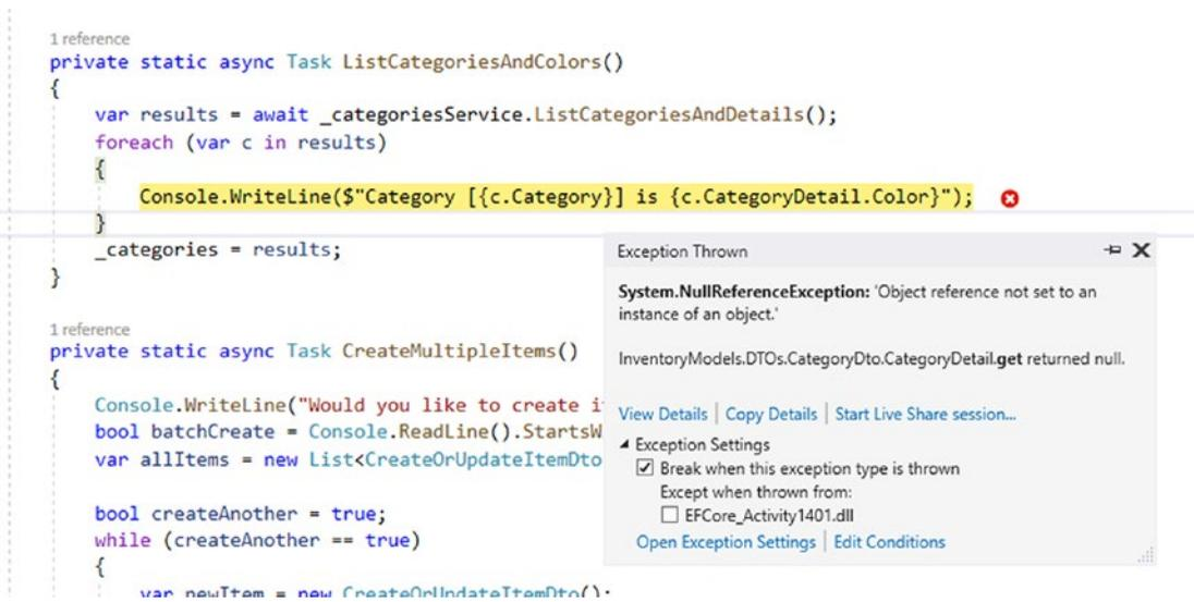
**Figure 14-1.** The additional category doesn't have any details, so the code as per Activity 13-1 encounters a null reference exception
