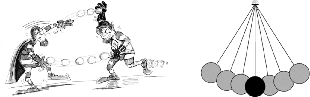
Figure 4.13: The simple frictionless pendulum is an analog system to the LC circuit in the absence of any electrical resistance.
