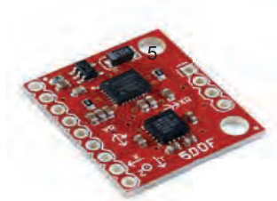
a) SparkFun IMU Analog Combo Board 5 Degrees of Freedom IDG500/ADXL335 SEN
