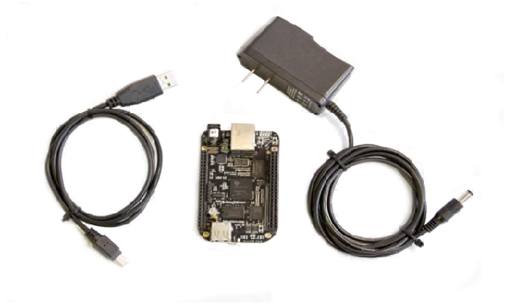
Figure 1.4: BeagleBone power source. (Photo courtesy of J. Barrett [2015], Closer to the Sun International).
