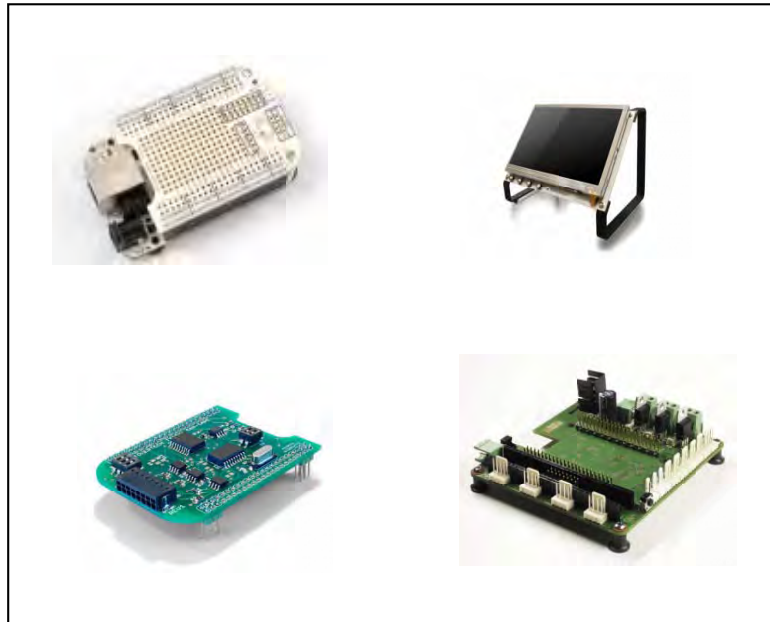
Figure 1.3: BeagleBone Capes: (Top left) prototype Cape; (top right) Liquid Crystal Display LCD7 Cape—Figures used with permission of Circuitco ( www.circuitco.com ); (bottom left) Controller Area Network Cape; (bottom right) motor control Cape—Figures used with permission of Circuitco ( www.circuitco.com ).
