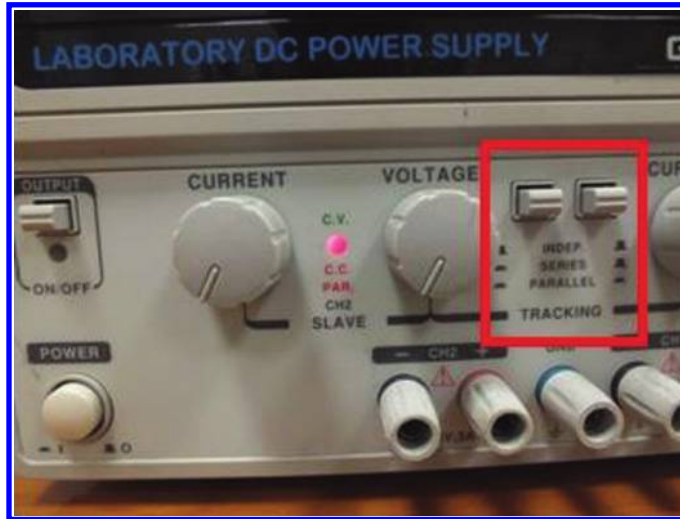
Figure 2.26: Buttons to set the operating mode of the PS.
