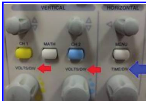
Figure 4.53: Each channel has its own VOLTS/DIV control. There is only one TIME/DIV control.
