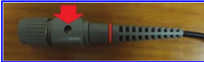
Figure 4.19: Probes have a small variable capacitor for compensation purposes. This is the variable capacitor of Fig. 4.13.
