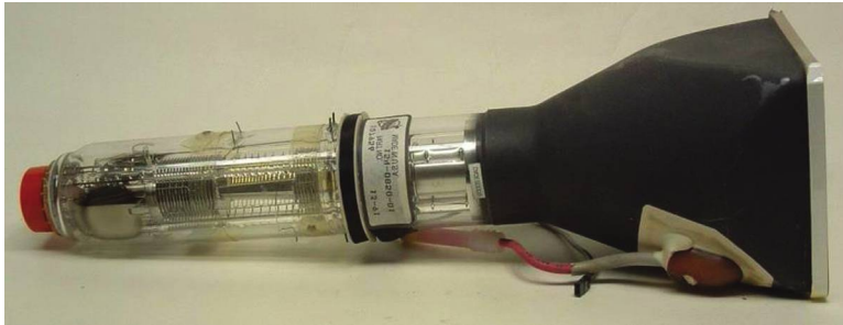
Figure 4.3: CRT of an analog oscilloscope.
