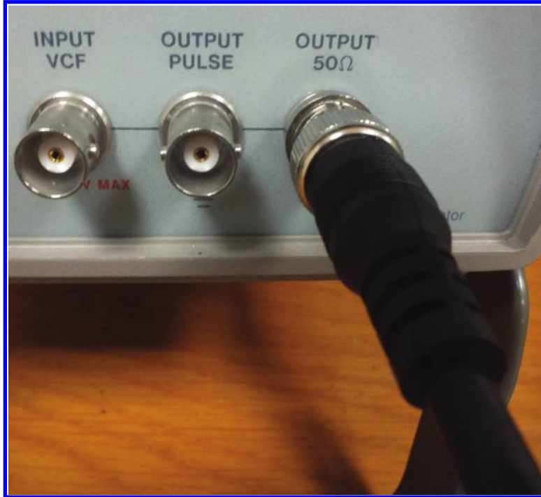
Figure 3.26: Output cable is connected to the 50 \Omega output.
