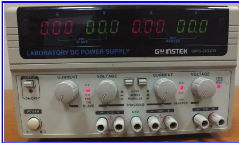
Figure 2.24: CH 1 and CH 2 have an ammeter and voltmeters in order to show the output current and voltage.
