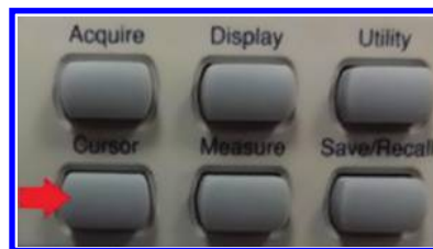
Figure 4.77: Manual measurement of settling time with cursors.
