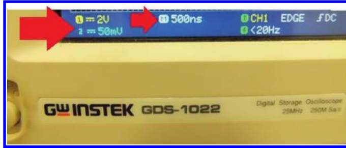
Figure 4.54: VOLTS/DIV for channel 1 is 2 V and for channel 2 is 50 mV. Value of TIME/DIV (for both channels) is 500 ns.
