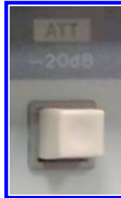
Figure 3.10: When you push this button, the output is attenuated by a factor of 10.
