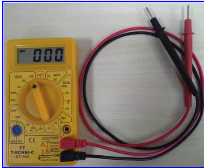
Figure 1.18: Put the selector in the DCV section.
