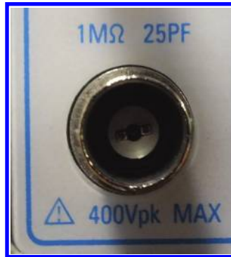
Figure 4.11: Values of R and C for input of NETES NS-2025C analog oscilloscope. R = 1\text{ M}\Omega and C = 25\text{ pF} .
