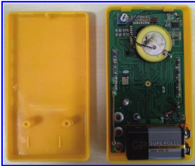
Figure 1.60: Open the back case in order to change the battery of DMM. Before opening the case, ensure that no external voltage enters the DMM circuit.
