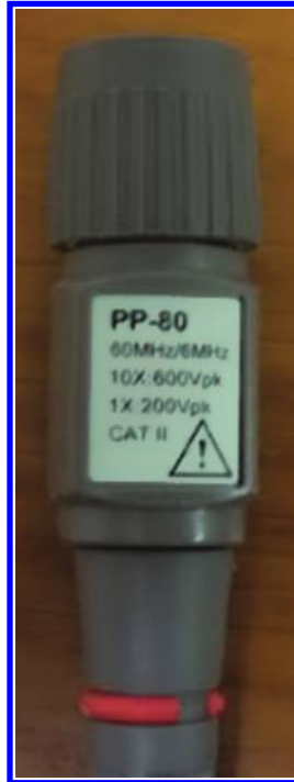
Figure 4.20: Maximum measurable frequency voltage is written on the probe label.
