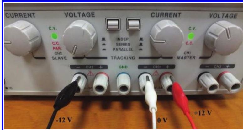
Figure 2.32: The series also could be used to obtain symmetric voltages. 0 V is taken from the negative output of channel 1.
