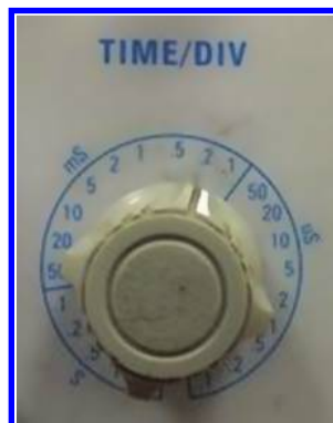
Figure 4.38: TIME/DIV control of NETES NS-2025C model analog oscilloscope.
