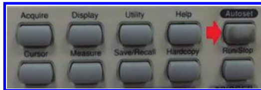
Figure 4.71: Autoset button could show the waveform on the screen automatically.
