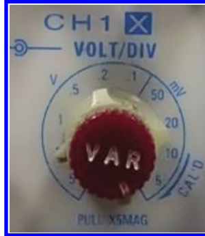
Figure 4.35: VOLTS/DIV control for channel 1 of NETES NS-2025C model analog oscilloscope. The red button on the VOLTS/DIV control of analog oscilloscopes must be always turned all the way clockwise, otherwise your measurement will be worthless.
