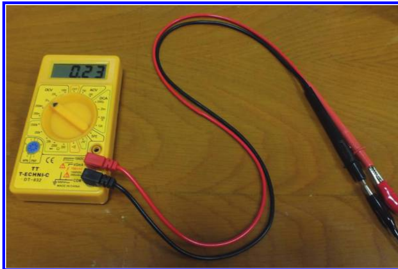
Figure 3.36: Measurement of the output DC value. Note that the DMM must be in the DC voltage measurement mode.
