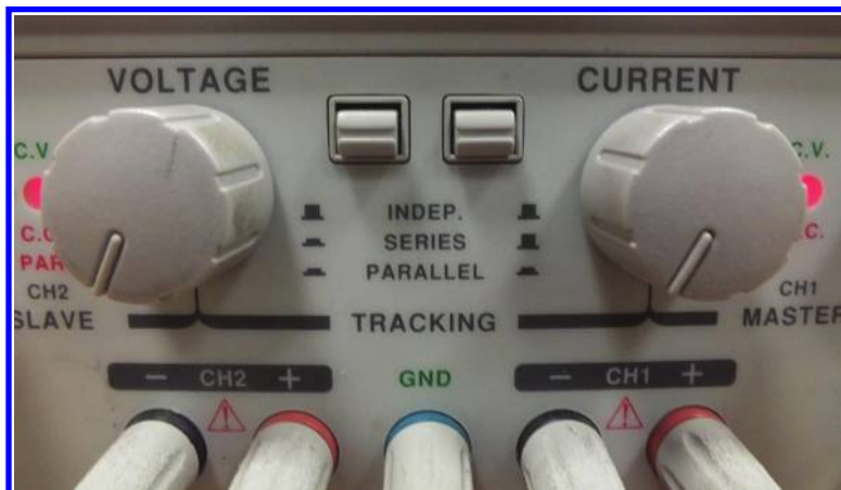
Figure 2.27: Close up of the mode selection unit of PS.
