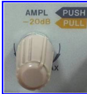
Figure 3.32: Amplitude knob. This knob controls the amplitude of the output waveform.
