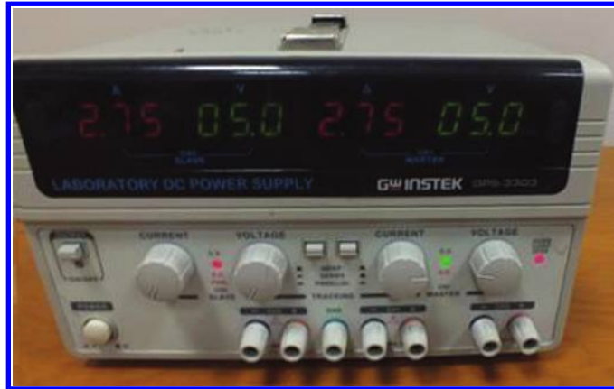
Figure 2.30: The maximum output is set to 2.75\text{ A} + 2.75\text{ A} = 5.5\text{ A} .
