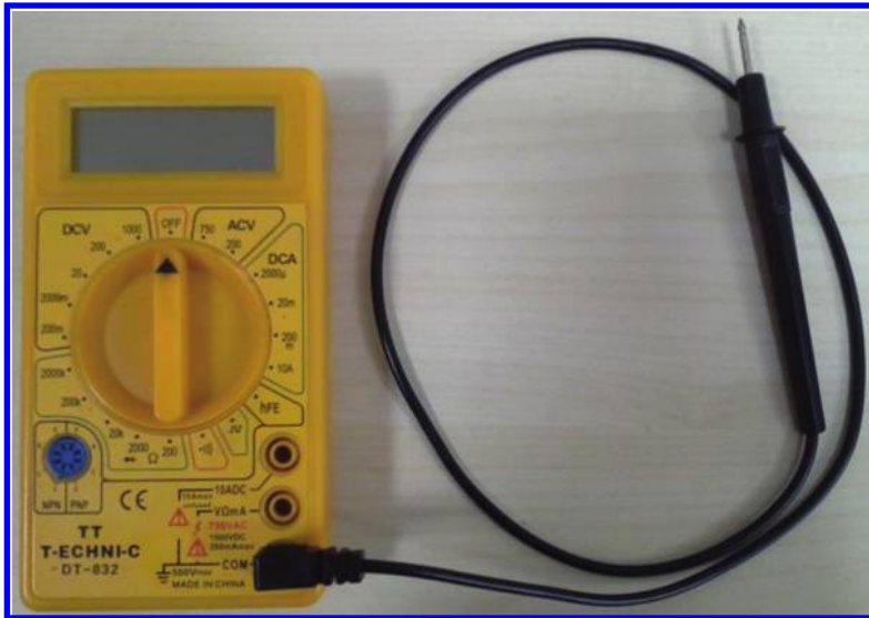
Figure 1.16: Black probe is always connected to the COM jack.
