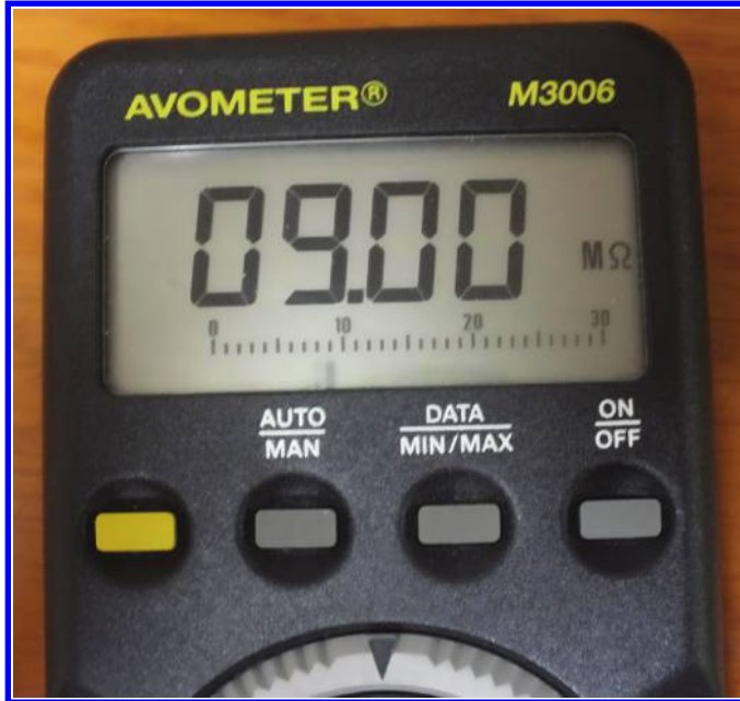
Figure 4.18: Measurement of probe resistor ( R_{\text{probe}} ) in the x10 case. R_{\text{probe}} = 9 \text{ M}\Omega .
