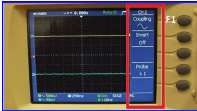
Figure 4.56: Type of coupling is set with the F1 button.
