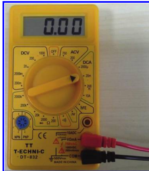
Figure 1.29: The COM and V \Omega mA is used for measurement of currents up to 20 \text{ mA} . The mode selector is in the 20 \text{ mA} state.
