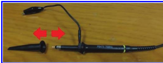
Figure 4.23: Taking out the probe cap.
