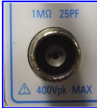
Figure 4.21: The NETES NS-2025C analog oscilloscope could accept voltage with peak values of less than 400 V.
