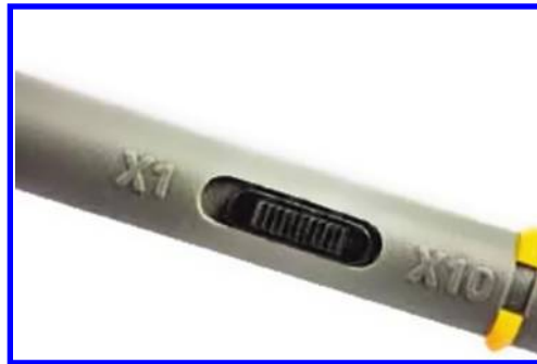
Figure 4.15: Oscilloscope probes usually have a switch on them.
