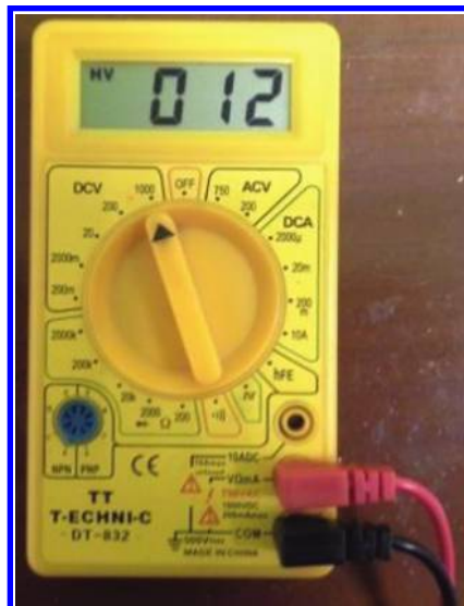
Figure 1.19: Selector is in the 1000 V mode. Reading is 12 V.
