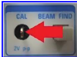
Figure 4.25: Calibration point of NETES NS-2025C model oscilloscope.
