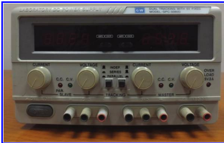
Figure 2.2: A three-channel PS. Two variable channels and one fixed (+5 V) channel.
