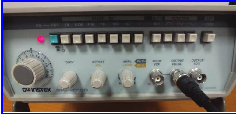
Figure 3.47: The output cable is connected to the pulse output of the FG.
