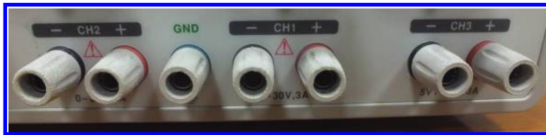
Figure 2.20: Output jacks of GW INSTEK GPS-3303. Protective earth is shown with GND label.
