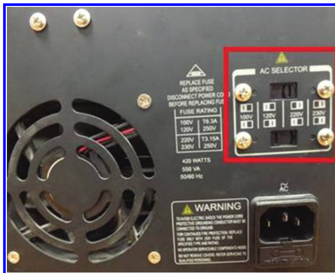
Figure 2.7: The AC selector switch must be set according to the grid voltage.
