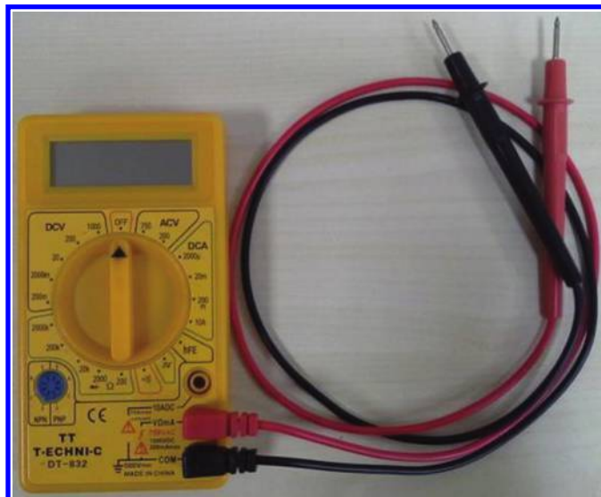
Figure 1.17: Connect the red probe to V \Omega mA.
