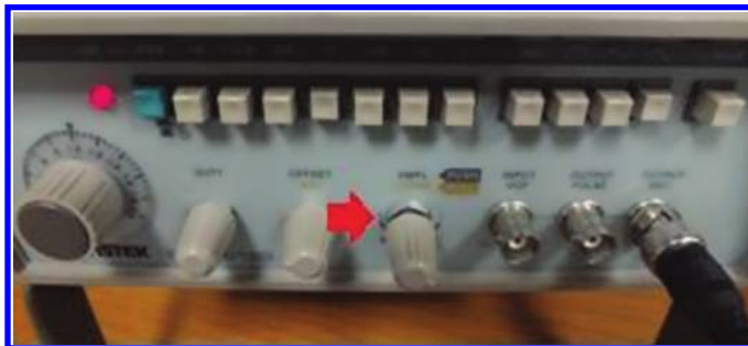
Figure 3.50: When you pull out the amplitude knob, the -20 dB activates.
