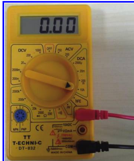
Figure 1.31: The COM and V \Omega mA is used for measurement of currents up to 10 A. The mode selector is in the 10 A state.
