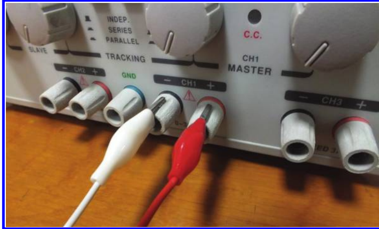
Figure 2.11: Using alligator clips for connection of the PS to the external circuit is NOT recommended.
