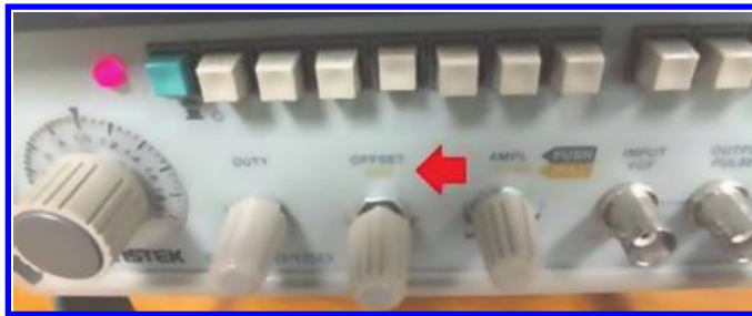
Figure 3.35: Pull out the offset knob in order to activate it.
