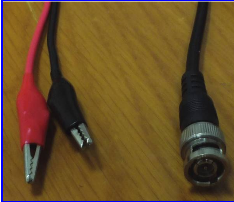
Figure 3.4: Output cables of FG have a BNC connector on one end and alligator clips on the other end.
