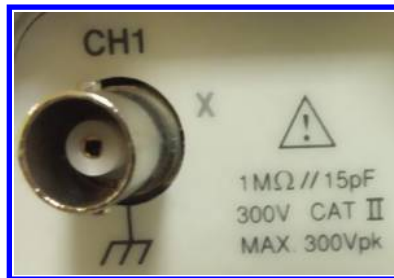
Figure 4.22: The GW INSTRON GDS-1022 digital oscilloscope could accept voltage with peak values of less than 300 V.
