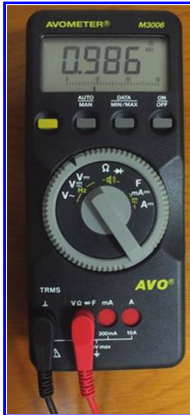
Figure 3.30: Output frequency is 0.986 kHz or 986 Hz.
