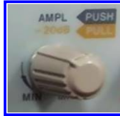
Figure 3.9: When you pull this knob, the output is decreased by a factor of 10.
