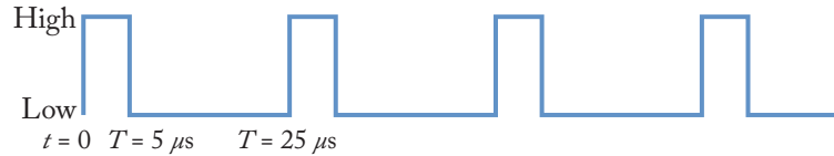
Figure 3.19: Duty ratio is D = \frac{5 \mu s}{25 \mu s} = 0.2 or 20%.
