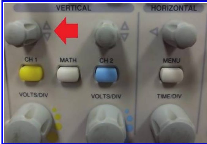
Figure 4.62: Channel 1 vertical control.
