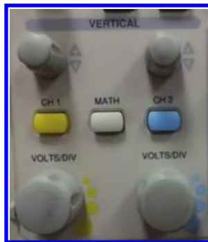
Figure 4.36: VOLT/DIV control of GW INSTEK GDS-1022 model digital oscilloscope.
