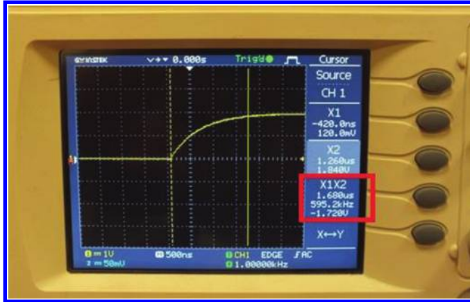
Figure 4.83: Time and voltage difference between the points which intersect the two cursors. The intersections are shown with red stars.
