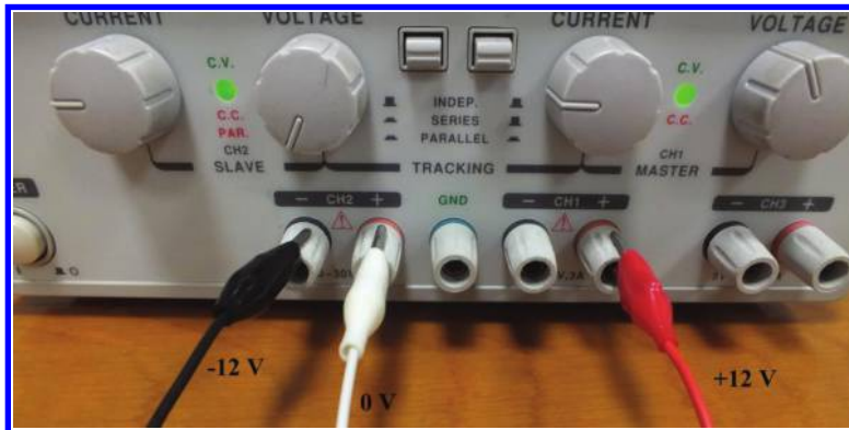
Figure 2.33: 0 V can be taken from the positive output of channel 2.
