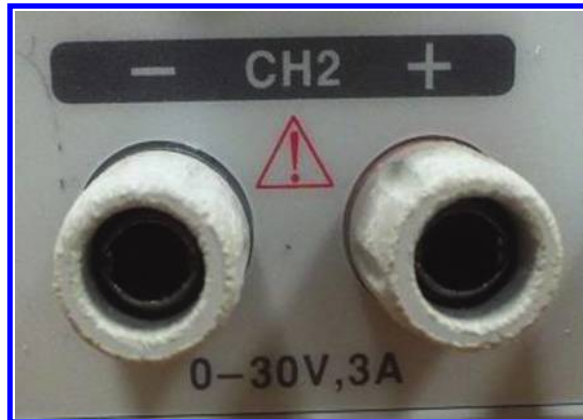
Figure 2.22: Channel 2 of GW INSTEK GPS-3303. According to the label, this channel could provide 0–30 V with maximum current of 3 A.
