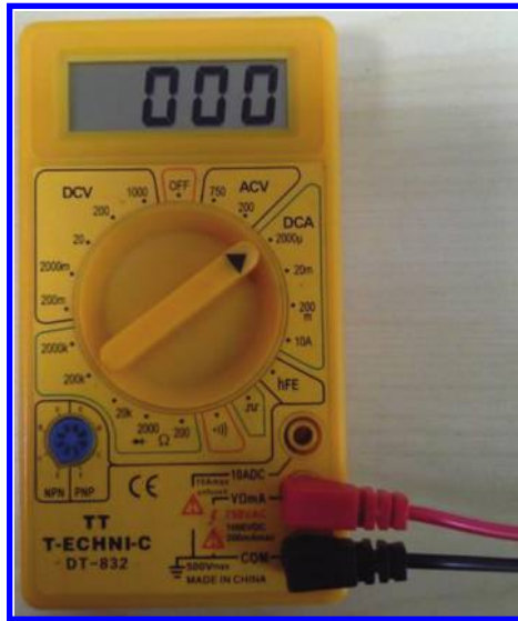
Figure 1.28: The COM and V \Omega mA is used for measurement of currents up to 2000 \mu\text{A} = 2 \text{ mA} . The mode selector is in the 2000 \mu\text{A} state.
