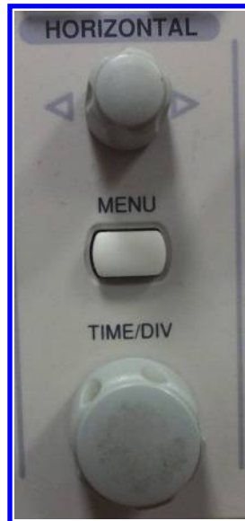
Figure 4.39: TIME/DIV control of GW INSTEK GDS-1022 model digital oscilloscope.
