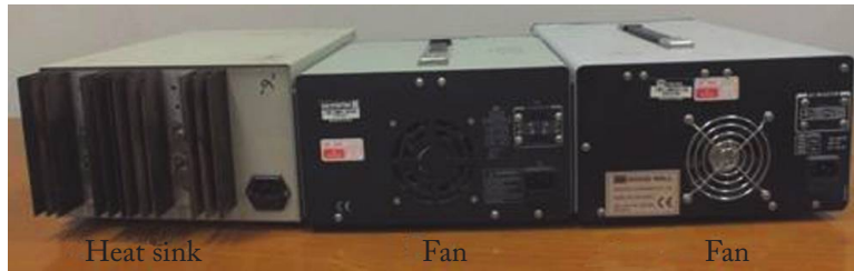
Figure 2.6: Use of fan and heatsink for decreasing the temperature of power transistors of the PS.
