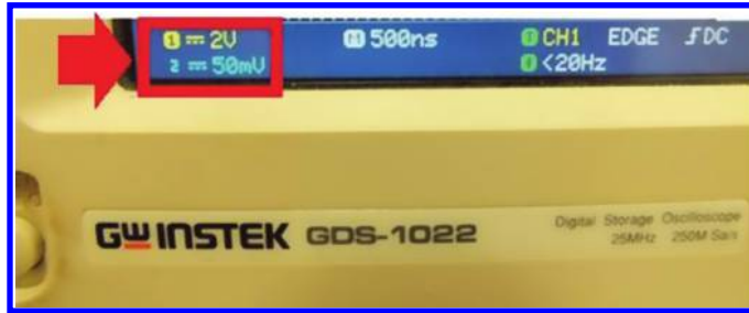
Figure 4.60: Coupling of channel 1 and 2 is DC.
