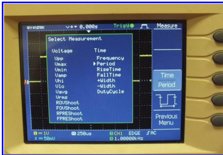
Figure 4.74: Different types of measurements which you can do with GW INSTEK GDS-1022.
