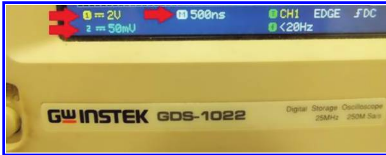
Figure 4.41: The value of VOLTS/DIV and TIME/DIV is shown at the bottom of the screen. VOLTS/DIV for channel 1 is 2 V and for channel 2 is 50 mV. TIME/DIV is 500 ns.
