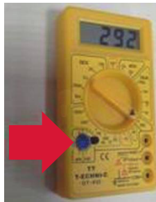
Figure 1.52: You can use the short circuit mode of the DMM in order to see whether two points of the PCB are connected together or not.
