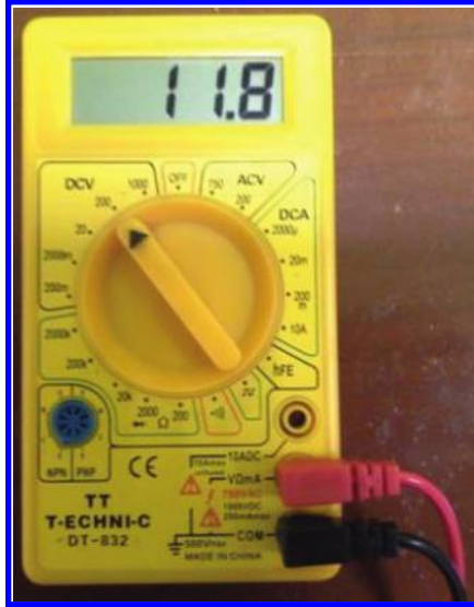
Figure 1.21: Selector is in the 200 V mode. Reading is 11.8 V.
