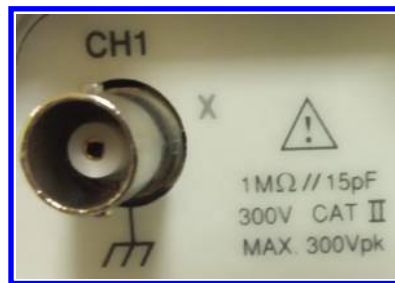
Figure 4.12: Values of R and C for input of GW INSTRUK GDS-1022 digital oscilloscope. R = 1\text{ M}\Omega and C = 15\text{ pF} .
