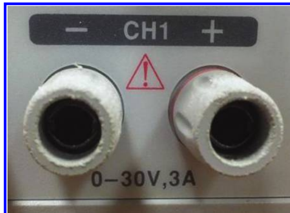
Figure 2.21: Channel 1 of GW INSTEK GPS-3303. According to the label, this channel could provide 0–30 V with maximum current of 3 A.
