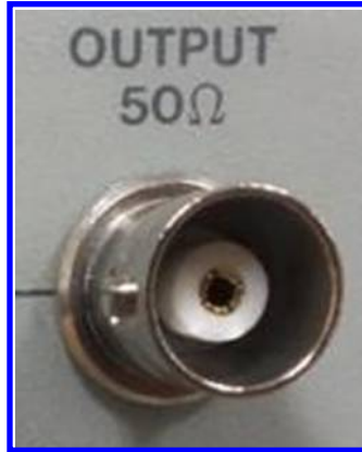
Figure 3.5: Generally, the output resistance of FGs is 50\ \Omega .
