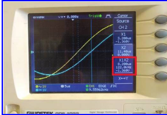
Figure 4.87: Measurement of time delay between the two waveforms.
