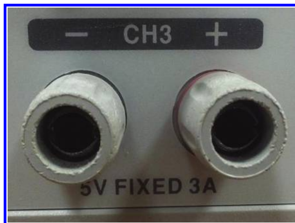
Figure 2.23: Channel 3 of GW INSTEK GPS-3303. According to the label, this channel could provide fixed 5 V with maximum current of 3 A.
