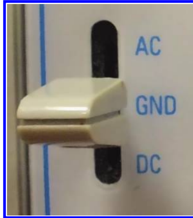
Figure 4.44: NETES NS-2025C model analog oscilloscope coupling selector.
