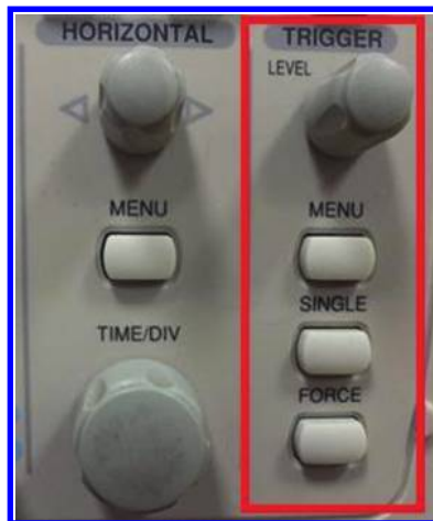
Figure 4.67: Use the LEVEL knob to stabilize a moving waveform.
