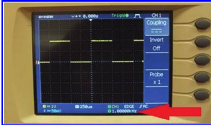
Figure 4.66: Frequency of periodic signals are shown in the bottom of the screen.
