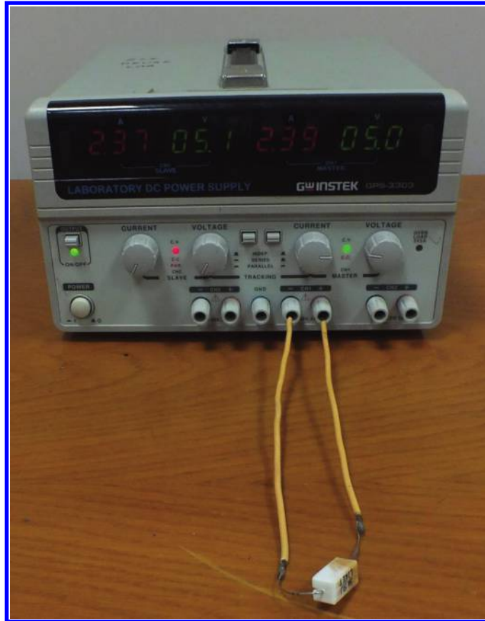
Figure 2.28: When output is taken from the master channel, the load current is divided almost equally between the two channels.
