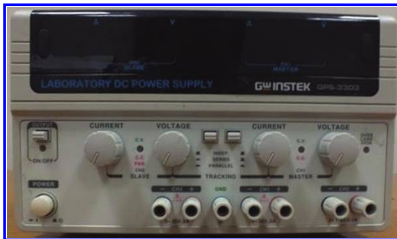
Figure 2.1: A three-channel PS. This model has two variable channels and one fixed +5 V output. Generally, the PSs are equipped with voltmeters and ammeters.
