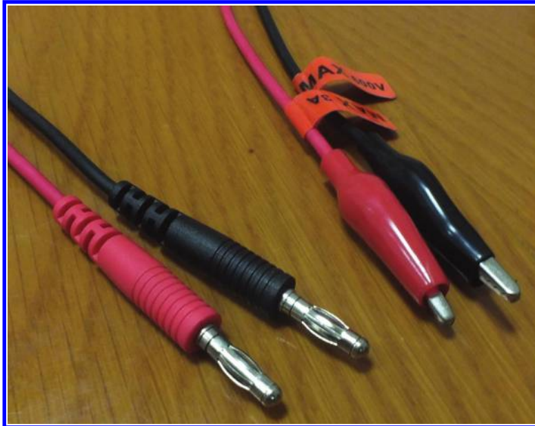
Figure 2.9: PS output cables have a banana plug at one end and alligator clips at the other end.
