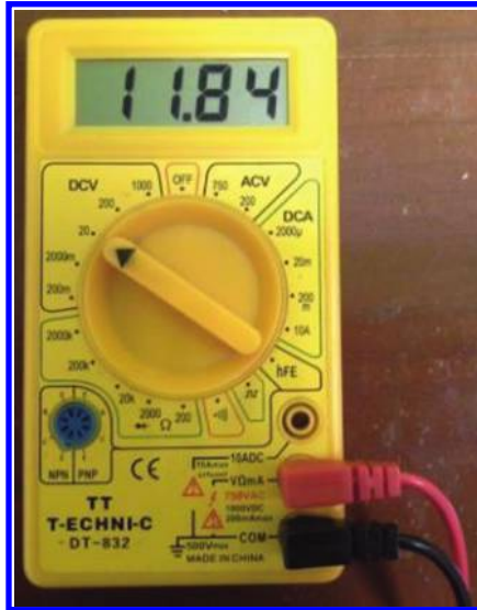
Figure 1.20: Selector is in the 20 V mode. Reading is 11.84 V.
