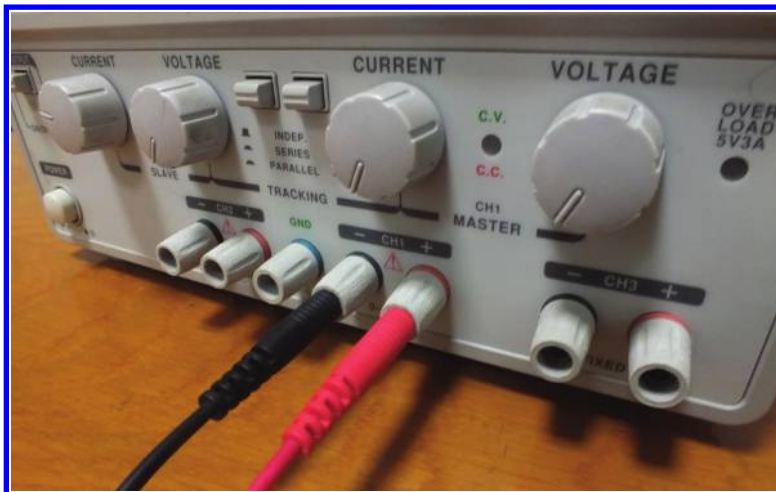
Figure 2.10: Connection of the output cable to the PS. The output jack of the PS is designed for banana plugs.
