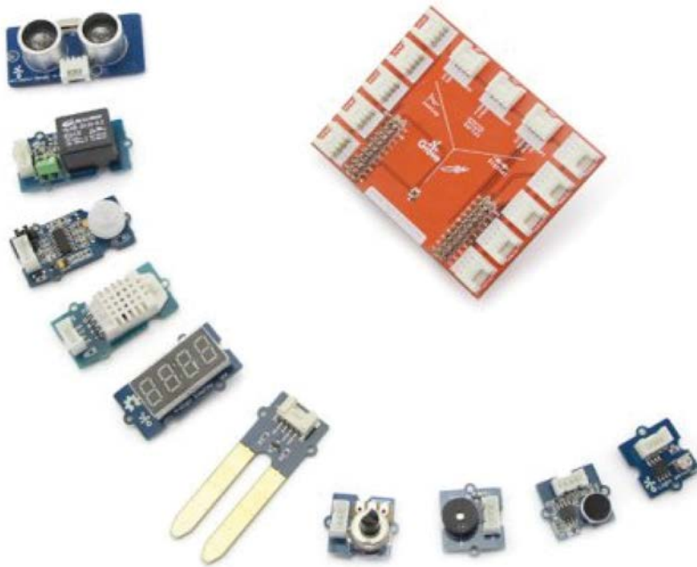
Figure 3.39: Grove Starter Kit for LaunchPad ( www.seeedstudio.com ). Illustrations used with permission of Texas Instruments ( www.TI.com ).
