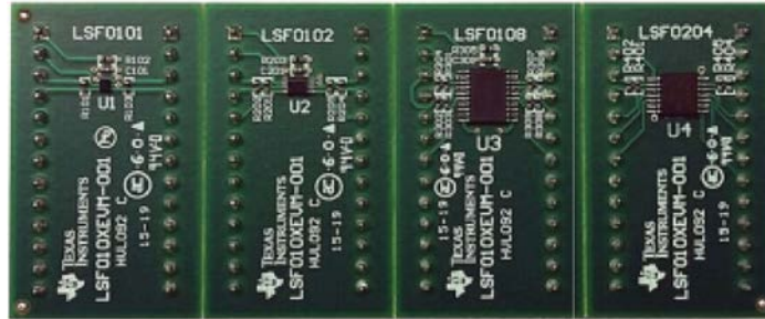
Figure 3.3: LSF010XEVM-001 Bi-Directional Multi-Voltage Level Translator Evaluation Module (LSFEVM). Image used with permission of Texas Instruments ( www.ti.com ).
