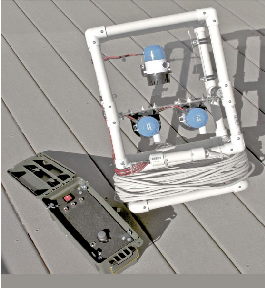
Figure 11.15: ROV fully assembled. (Photo courtesy of J. Barrett, Closer to the Sun International.)
